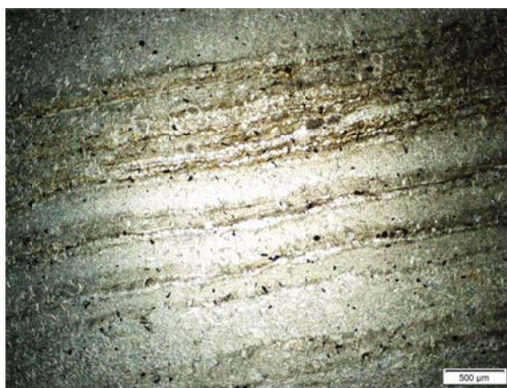
Figure 18.40 Utah: Limestone Example B Thin Section Under Plane-Polarized Light, 2x magnification
