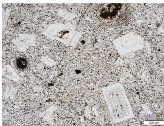
Figure 18.27 Lockwood, Nevada: Basalt, Andesite, Rhyolite Example Thin Section Under Plane-Polarized Light, 2x magnification
