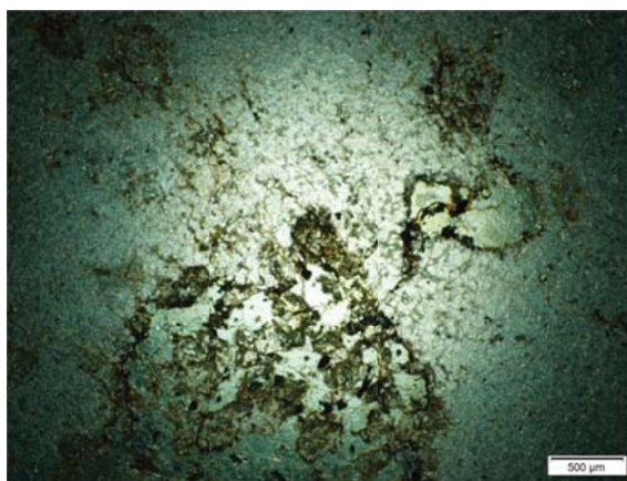
Figure 18.2 Gardner, California: Mudstone Example Thin Section Under Plane-Polarized Light, 2x magnification
