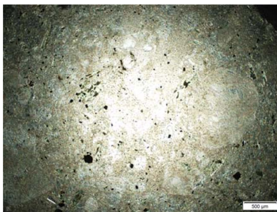
Figure 18.38 Utah: Limestone Example A Thin Section Under Plane-Polarized Light, 2x magnification
