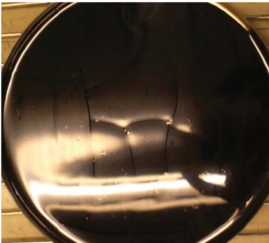
Figure 10.1 Example of Cracked Pan-Aged PG64-28 Binder Aged at 50°C for 60 days
