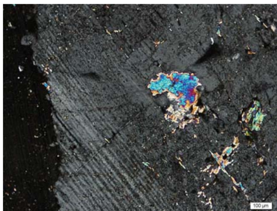
Figure 18.23 Morrison, Colorado: Muscovite (Mica Gneiss) Thin Section Under Cross-Polarized Light, 10x magnification
