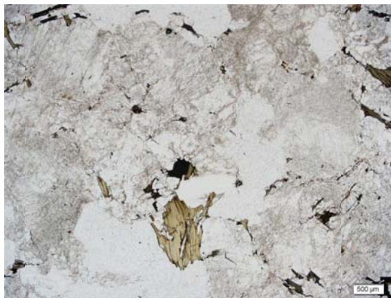
Figure 18.21 Morrison, Colorado: Mica Gneiss Example Thin Section Under Plane-Polarized Light, 2x magnification
