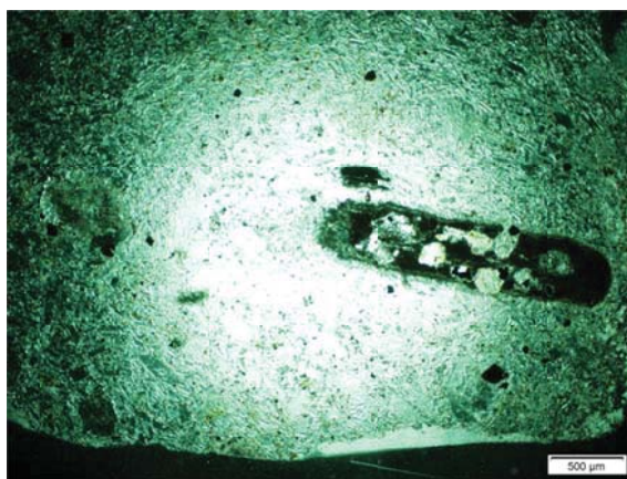
Figure 18.70 WesTrack 1997: Basalt to Andesite Example C Thin Section Under Plane-Polarized Light, 2x magnification
