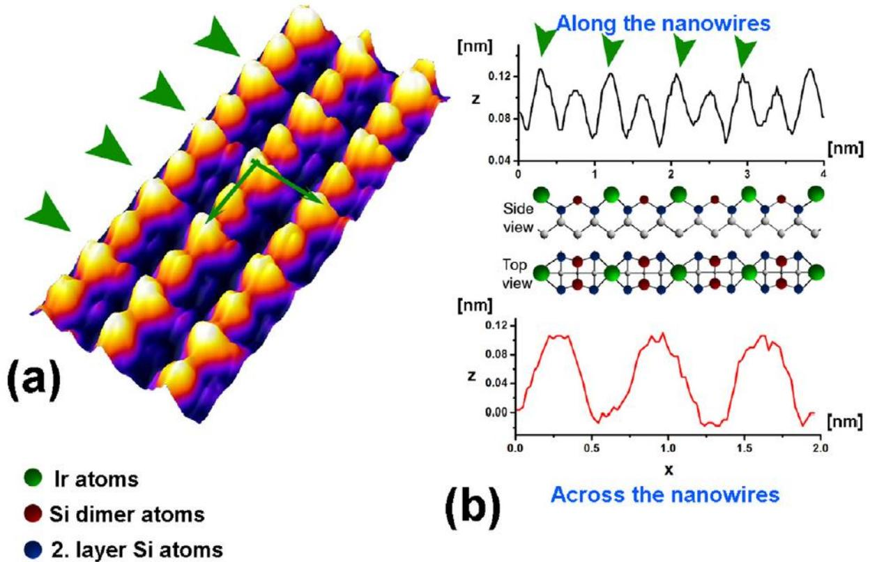
**Figure 5. 11** (a)  $4.5 \text{ nm} \times 2 \text{ nm}$  3-D STM image of the Ir-silicide nanowires,  $V = -1.0 \text{ V}$ ,  $I = 0.5 \text{ nA}$ . (b) Top (bottom) shows a line scan along (across) the nanowires. A schematic model for the Ir-silicide nanowires is presented between the line scans.
