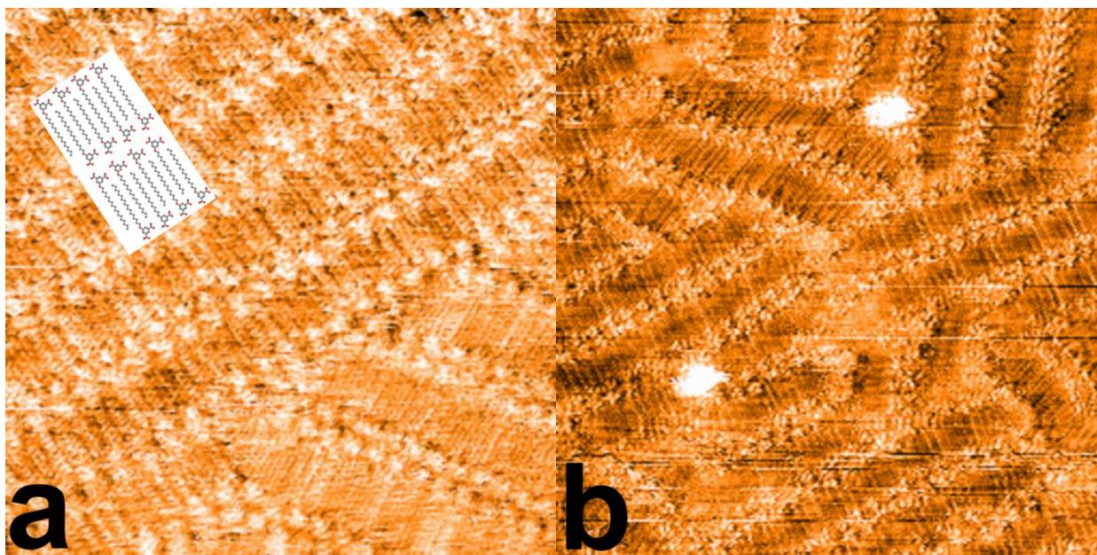
**Figure 3.2** (a)  $19.1 \text{ nm} \times 19.1 \text{ nm}$  STM image of 5-OIA on HOPG,  $V_{tip} = 0.88 \text{ V}$ ,  $I = 0.45 \text{ nA}$ . (b)  $25.2 \text{ nm} \times 25.2 \text{ nm}$  STM image of two Cu-TCPP molecules (two white blobs) adsorbed on 5-OIA modified HOPG surface,  $V_{tip} = 1.1 \text{ V}$ ,  $I = 0.6 \text{ nA}$ .
