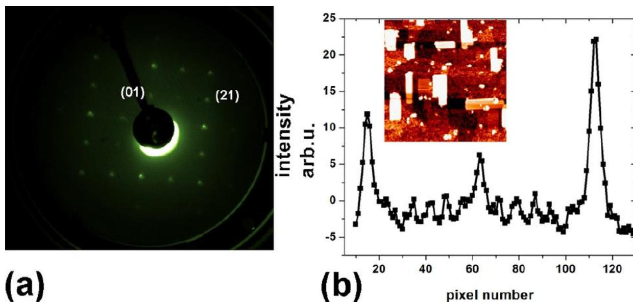
**Figure 5.9** (a) LEED intensity image after 0.125 *ML* of Ir deposition and annealing at 700°C. (b) Line scan of LEED image from (01) beam to (21) beam. The electron energy for the LEED pattern is 49 eV. Inset is the corresponding large-scale STM image of the surface.
