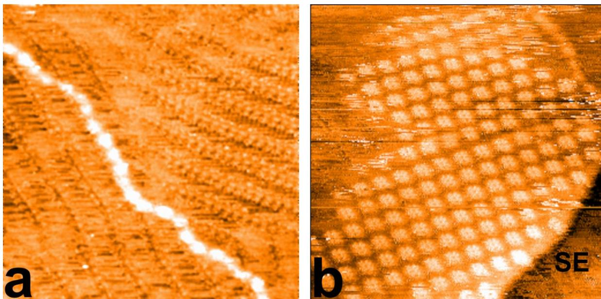
**Figure 3. 3** (a)  $29.4 \text{ nm} \times 29.4 \text{ nm}$  STM image of Cu-TCPP chain over 5-OIA head groups,  $V_{tip} = 1.2 \text{ V}, I = 0.7 \text{ nA}$ . (b)  $30.5 \text{ nm} \times 30.5 \text{ nm}$  STM image of Cu-TCPP 2-D patch building next to a step edge (denoted by SE),  $V_{tip} = 1.2 \text{ V}, I = 0.6 \text{ nA}$ .
