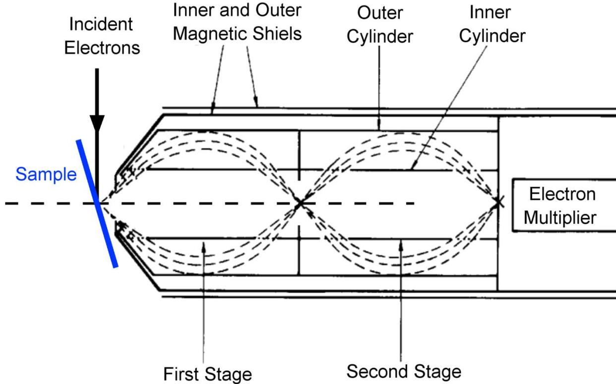
**Figure 2. 4** Schematic of AES setup with sample set at a grazing angle with respect to incident electrons.
