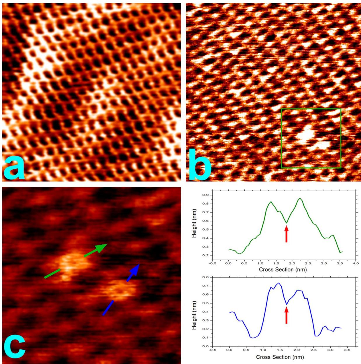
**Figure 4. 4** (a)  $5 \text{ nm} \times 5 \text{ nm}$  STM image of graphene over  $(6\sqrt{3})$  reconstruction  $V = -0.606 \text{ V}$ ,  $I = 0.508 \text{ nA}$ . (b)  $25 \text{ nm} \times 25 \text{ nm}$  STM image of Zn-Pc molecules on graphene  $V = -0.929 \text{ V}$ ,  $I = 0.777 \text{ nA}$ . (c)  $9 \text{ nm} \times 9 \text{ nm}$  STM image of highlighted region in (b),  $V = -0.929 \text{ V}$ ,  $I = 0.777 \text{ nA}$  and respective line scans across each of the Zn-Pc molecules.
