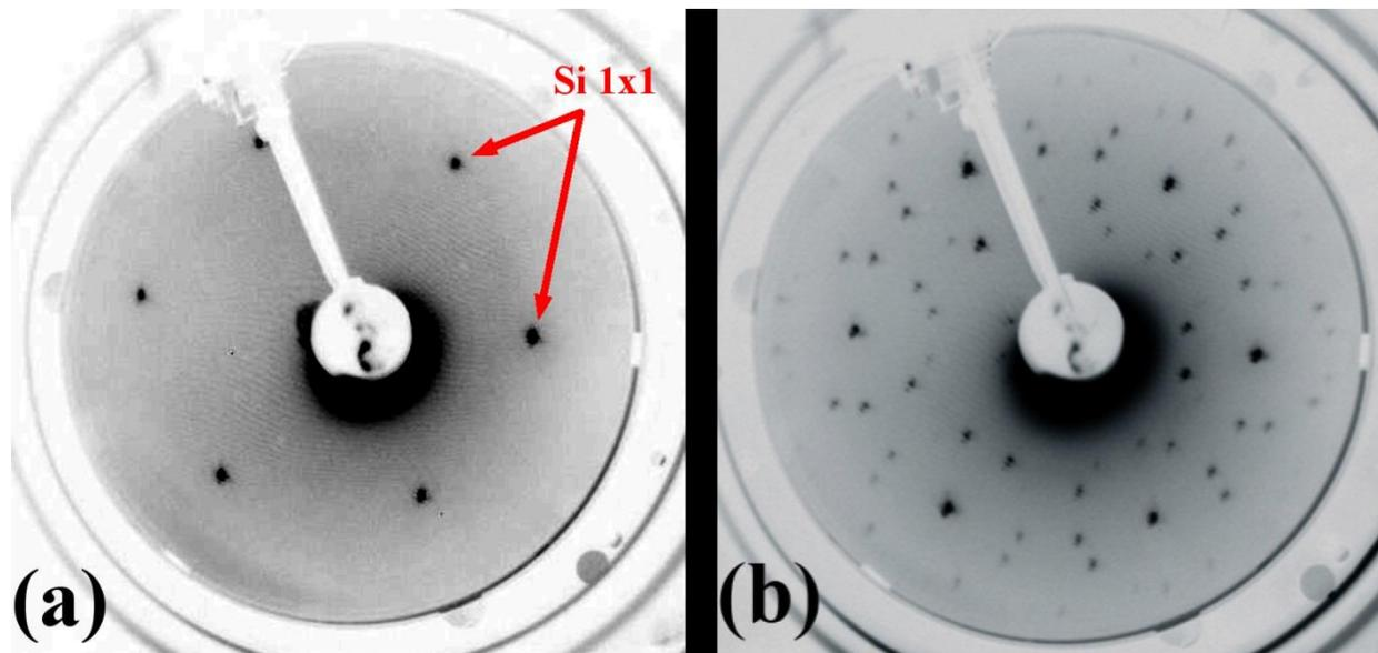
**Figure 5. 2** LEED pattern sequence after annealing at: (a)  $\sim 350^\circ\text{C} - 650^\circ\text{C}$  showing only a Si  $1 \times 1$  pattern, (b)  $\sim 750^\circ\text{C}$  with  $\sqrt{7} \times \sqrt{7} R19.1^\circ$  pattern.
