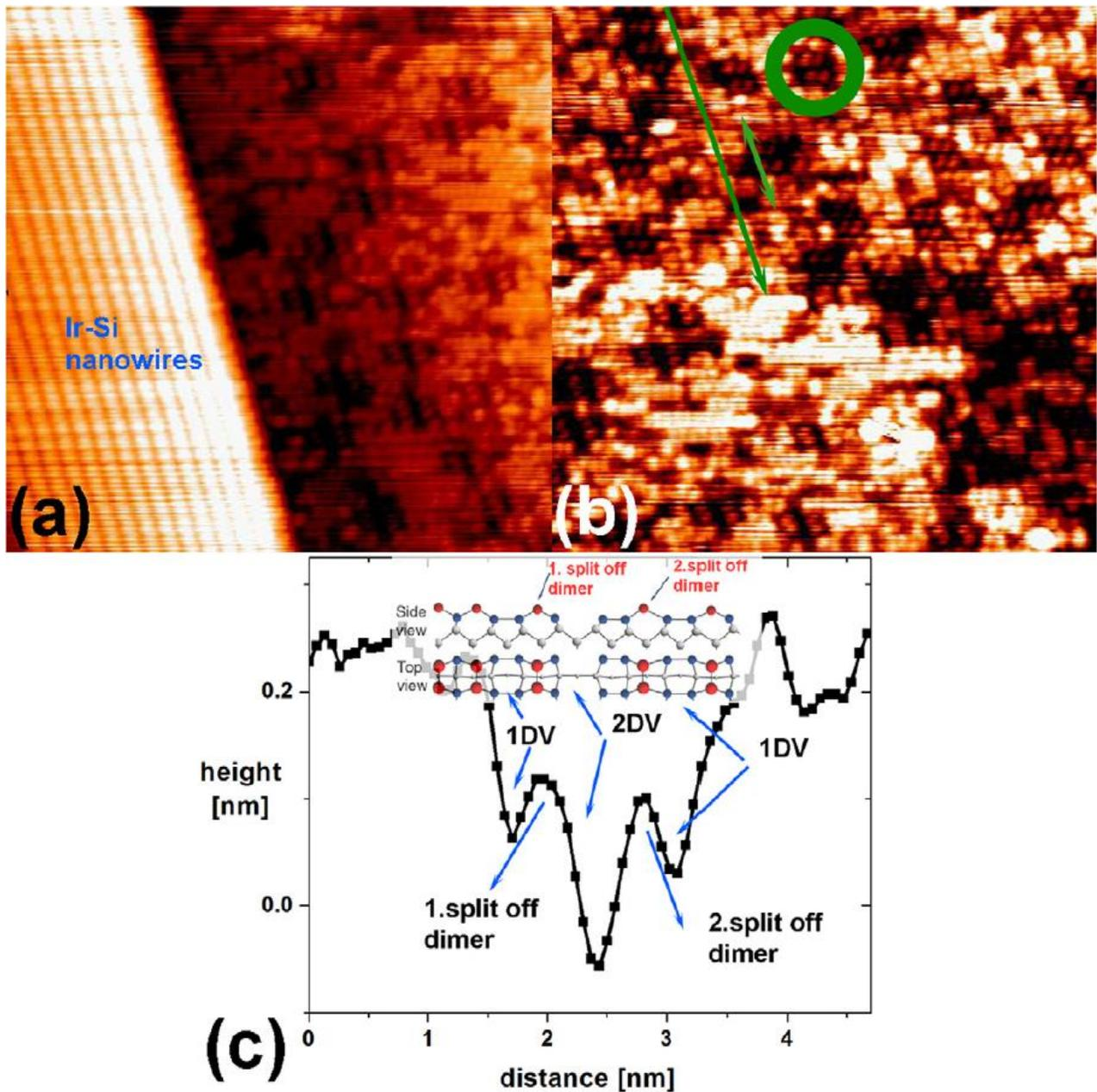
**Figure 5. 10** (a)  $25\text{ nm} \times 25\text{ nm}$  STM image showing both Ir-silicide terrace and Si(100) surface,  $V = -1.0\text{ V}$ ,  $I = 0.5\text{ nA}$ . (b)  $24\text{ nm} \times 24\text{ nm}$  STM image of the Ir modified Si(100) surface,  $V = -1.0\text{ V}$ ,  $I = 0.5\text{ nA}$ . The longer arrows indicates both the direction of Ir-silicide nanowires and dimer rows of Si(100). (c) Line scan over the shorter arrow presented with a model of the Si(100) terrace.
