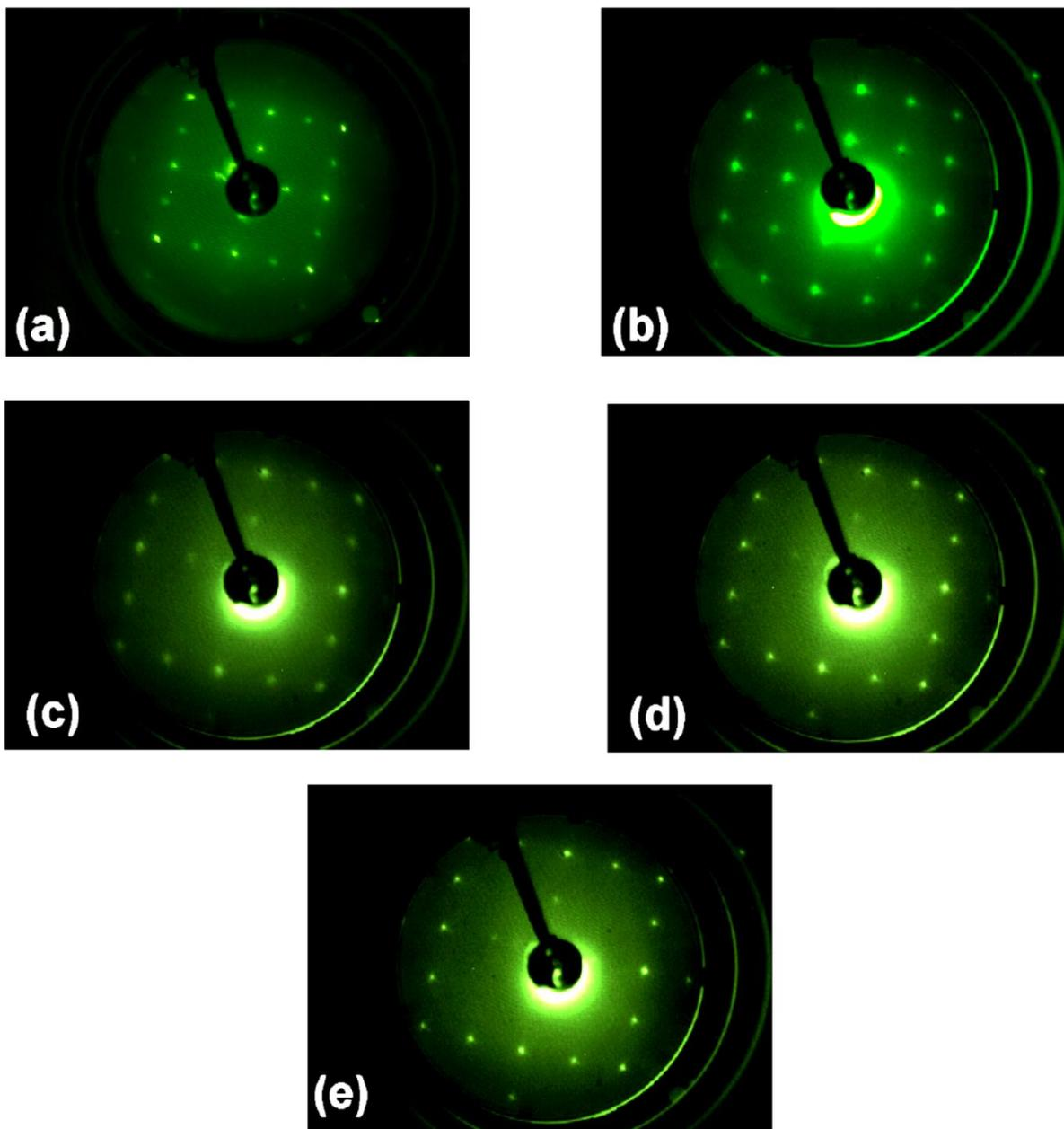
**Figure 5. 6** LEED intensity images of: (a) Clean Si(100)- $2 \times 1$  reconstructed surface, (b) Ir-modified Si(100) surface with a  $p(2 \times 2)$  pattern, (c,d,e) Surface after annealing at 800°C, 900°C, and 1000°C, respectively. The electron energy for all LEED images is 49 eV.
