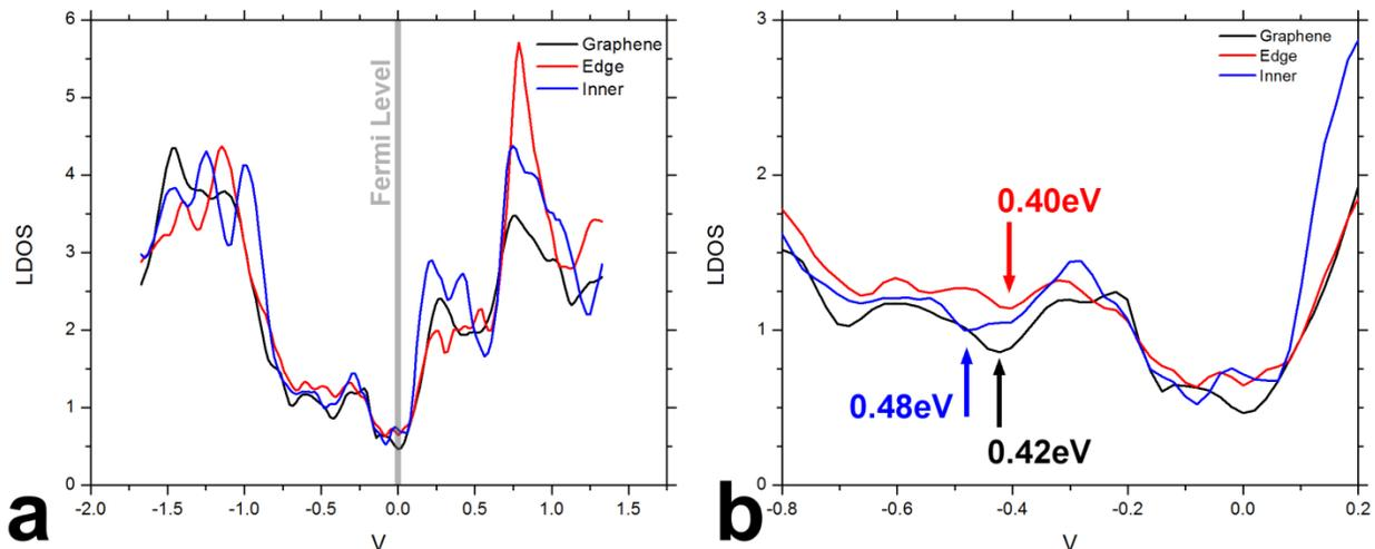
**Figure 4. 5** (a) LDOS comparison of the graphene surface, edge of the Zn-Pc molecule, inner-core of the Zn-Pc molecule. (b) Section of the same LDOS curves in (a), near the Dirac point  $\sim 0.42$  eV. Clear shifts of the Dirac point near the (edge/inner-core) of the Zn-Pc molecule are evidence of (n-doping/p-doping), respectively.
