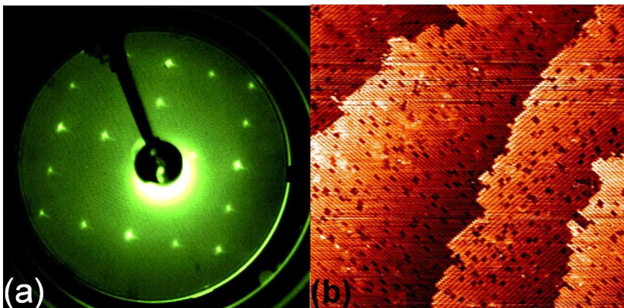
**Figure 5. 7** (a) LEED intensity image showing Si(100)- $2 \times 1$  returned after the Ir-modified sample was annealed at  $1250^{\circ}\text{C}$ . The electron energy is 49eV. (b)  $75 \text{ nm} \times 75 \text{ nm}$  STM image of the sample after the LEED image was taken,  $V = -1.75 \text{ V}$ ,  $I = 0.42 \text{ nA}$ .
