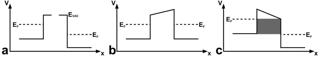
**Figure 2. 2** One-dimensional representation of potential barriers. (a) Non-interacting system with energy  $E_{VAC}$ . (b) Tip and sample in equilibrium with common Fermi energies and the difference between work functions is depicted as an electric field in the gap. (c) An applied voltage promotes tunneling between tip and sample where the energies in the gray area can contribute to tunneling.
