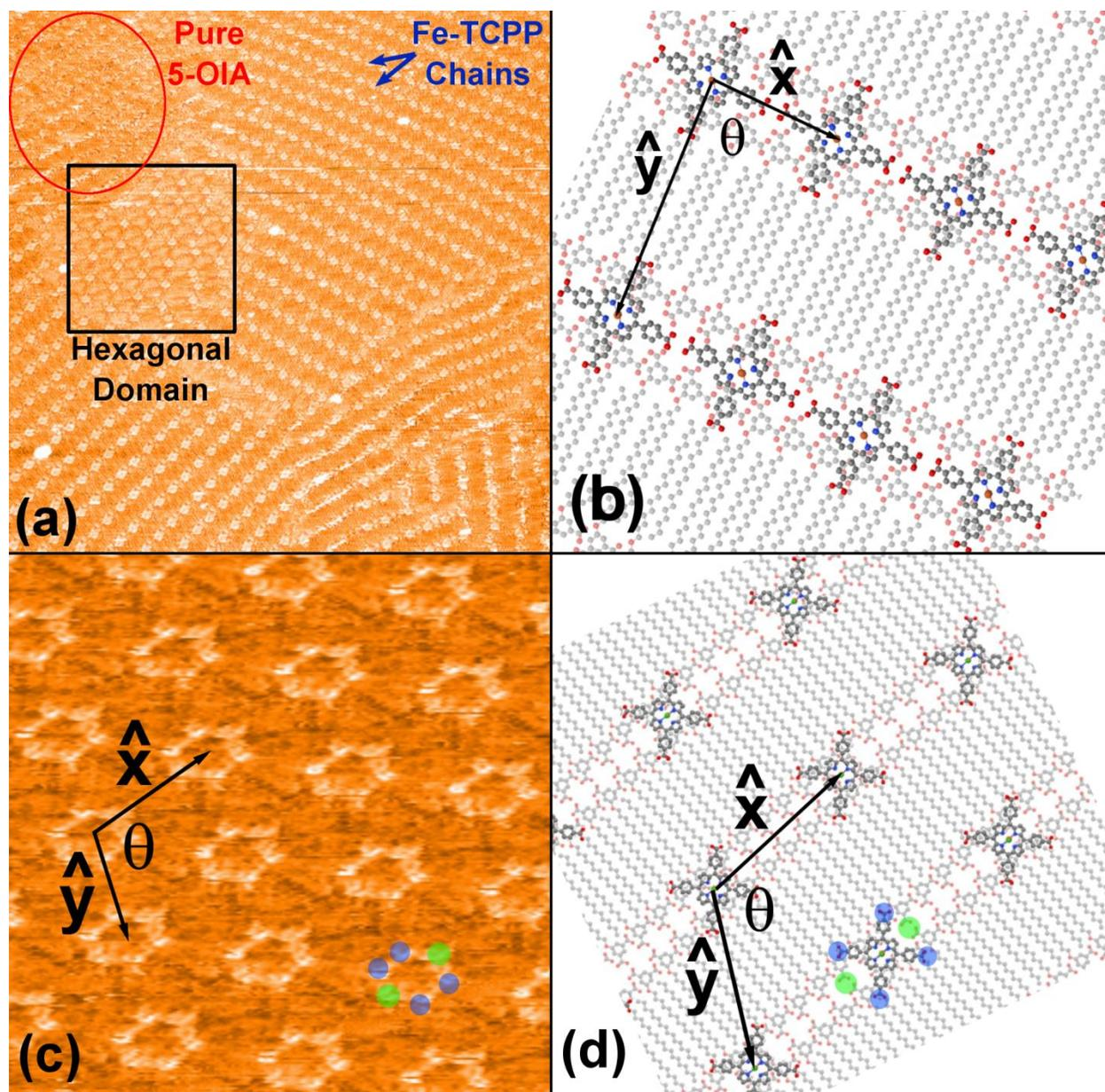
**Figure 3. 4** (a)  $100 \text{ nm} \times 100 \text{ nm}$  STM image of Fe-TCPP and 5-OIA domains,  $V_{tip} = 1.1 \text{ V}$ ,  $I = 0.4 \text{ nA}$ . (b) Schematic of Fe-TCPP chains over the head groups of 5-OIA. (c)  $30 \text{ nm} \times 30 \text{ nm}$  STM image of Fe-TCPP hexagonal domain,  $V_{tip} = 1.1 \text{ V}$ ,  $I = 0.18 \text{ nA}$ . (d) Schematic of hexagonal domains, again with Fe-TCPP over the head groups of 5-OIA.
