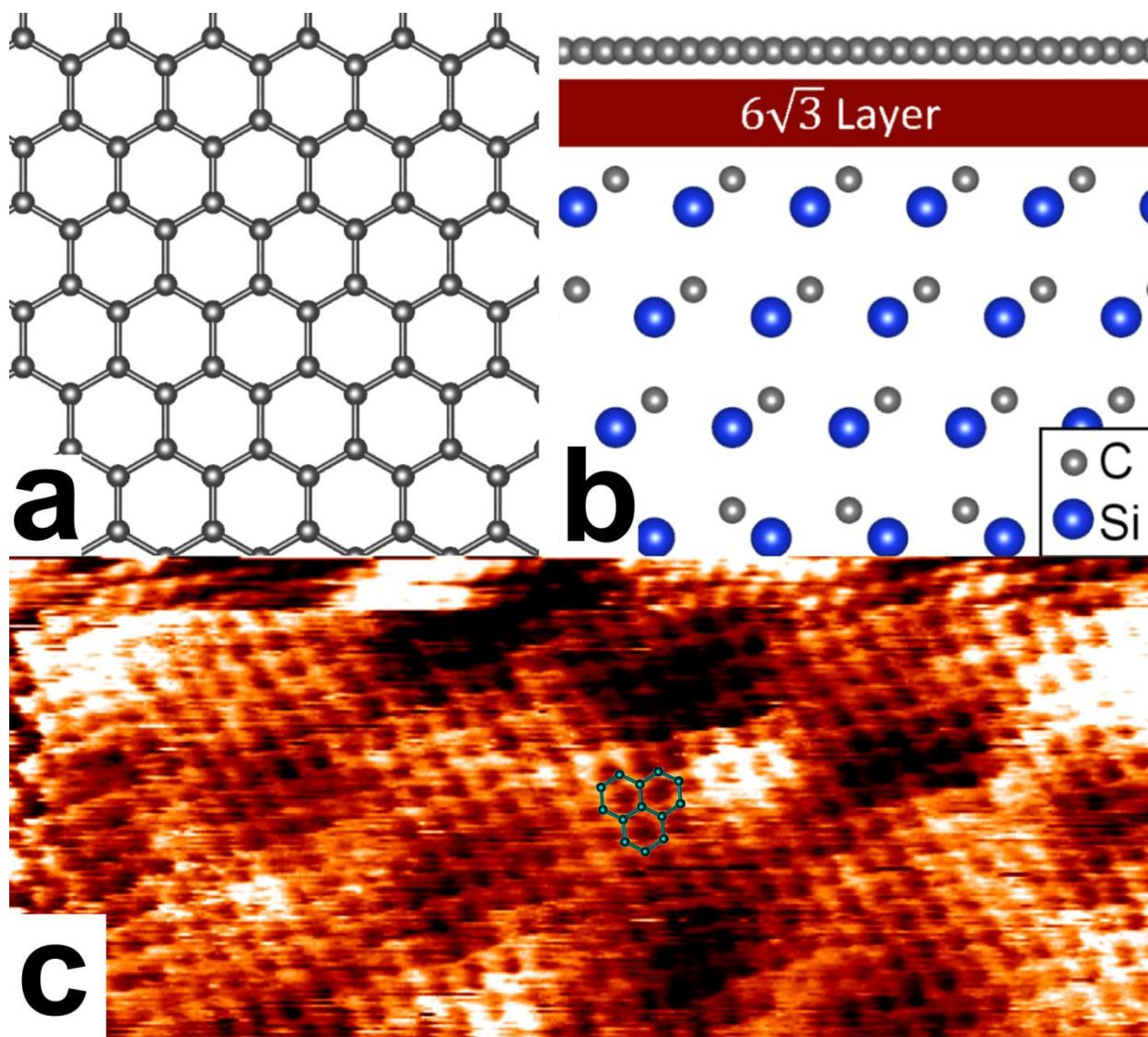
**Figure 4. 3** (a) Schematic of graphene. (b) Side-view schematic showing graphene atop the  $6\sqrt{3}$  buffer layer on a SiC substrate. (c)  $10\text{ nm} \times 3.75\text{ nm}$  STM image of graphene over  $(6\sqrt{3})$  reconstruction.  $V = -0.774\text{ V}$ ,  $I = 0.827\text{ nA}$ .
