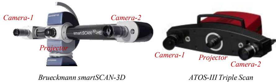
Figure 5.3 Top of the line Structured Light Scanners that employ sinusoidal illumination for recovering topographic information
