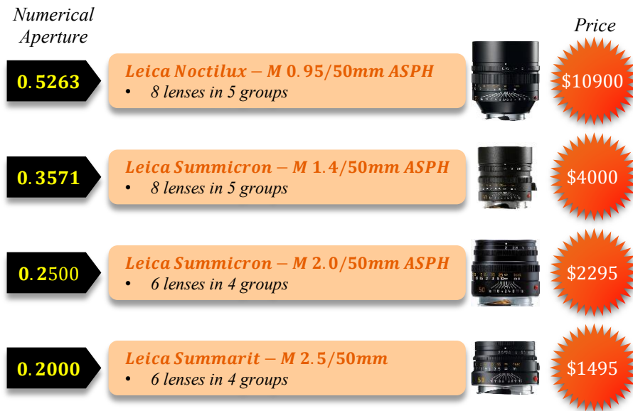
Figure 2.8 Resolution versus Cost tradeoff for 50mm Leica photographic lenses.
