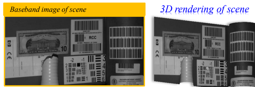
Figure 6.8 Texture-mapping the topographic map recovered in a canonical active stereo setup
