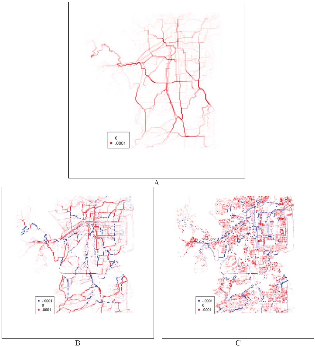
Figure 8.26: Comparison of heatmaps generated under the default parameters (A) and the parameter sweep runs with Max Speed set at 1000 m/5 min (B) and 8000 m/5 min (C).
