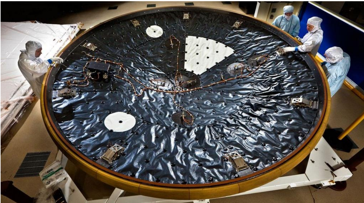
Figure 2.11. Interior of heat shield showing MEDLI hardware.†
