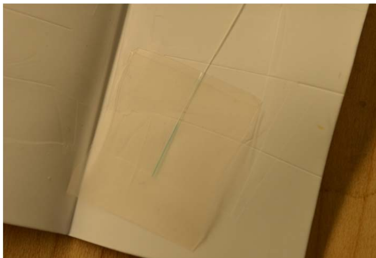
Figure 6-3: Embedded optical fiber sensing device within the Nafion ® membrane.
