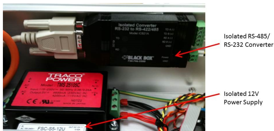
Figure B.6: Falcon Surface Equipment - the isolated RS-232/485 transceiver and isolated power supply that were added to the CPU box.
