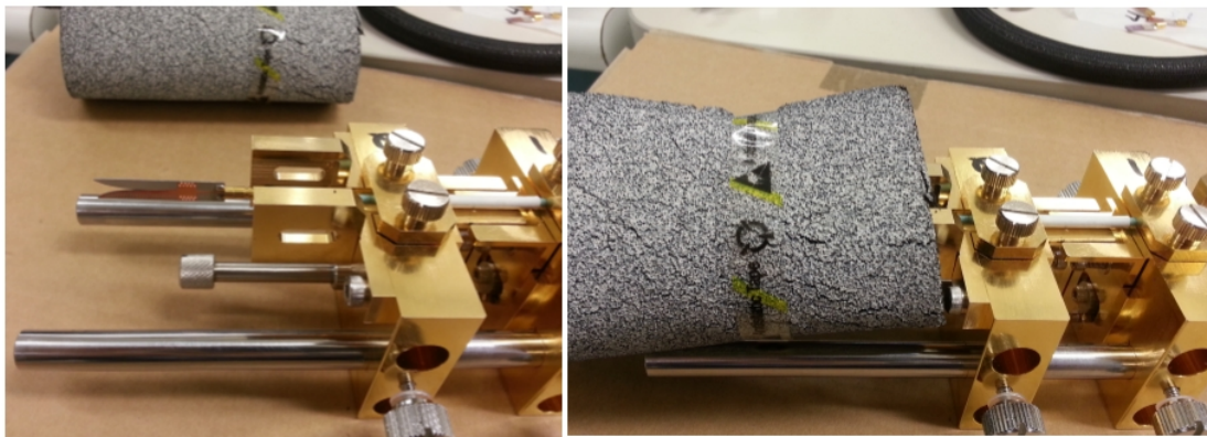
Figure 3.22: KPAF VNA setup (left) and with absorber around antenna (right) to prevent stray radiation from disturbing the S-parameter measurements.
