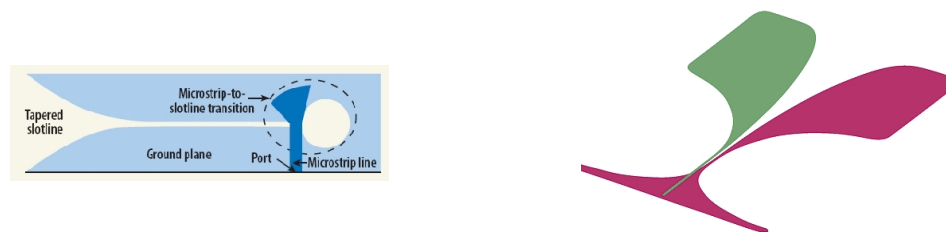
(a) Uniplanar Vivaldi antenna with microstrip feed. Light blue: top conducting plane. Dark blue: bottom conducting plane. Substrate not shown.
