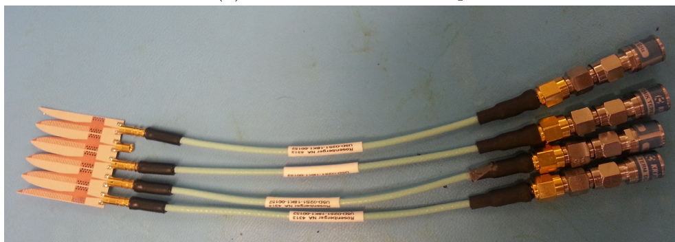
(e) Terminated unused ports
