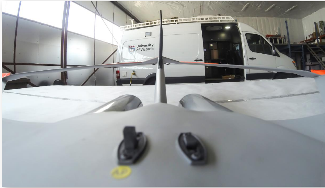
FIGURE 119 - CAMERA FIELD OF VIEW FOR CAPTURING AFT WING STRUCTURAL RESPONSE IN FLIGHT
