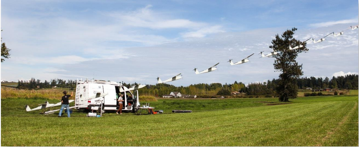
FIGURE 35 - AUTONOMOUS CATAPULT TAKEOFF TEST
