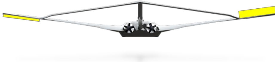
FIGURE 26 - RIGHT ROLLING MANEUVER USING AILERON DIFFERENTIAL
