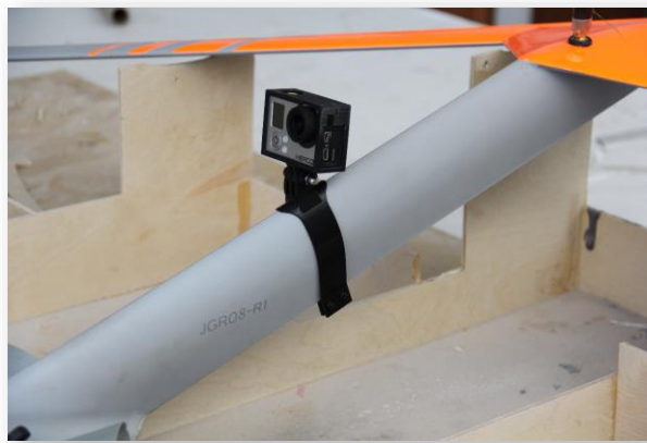
FIGURE 109 - CUSTOM BRACKET USED TO MOUNT GOPRO AND ADJUST CG
