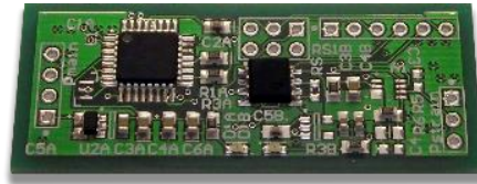
FIGURE 154 - CUSTOM DESIGNED PRINTED CIRCUIT BOARD FOR REMOTE STRAIN READINGS
