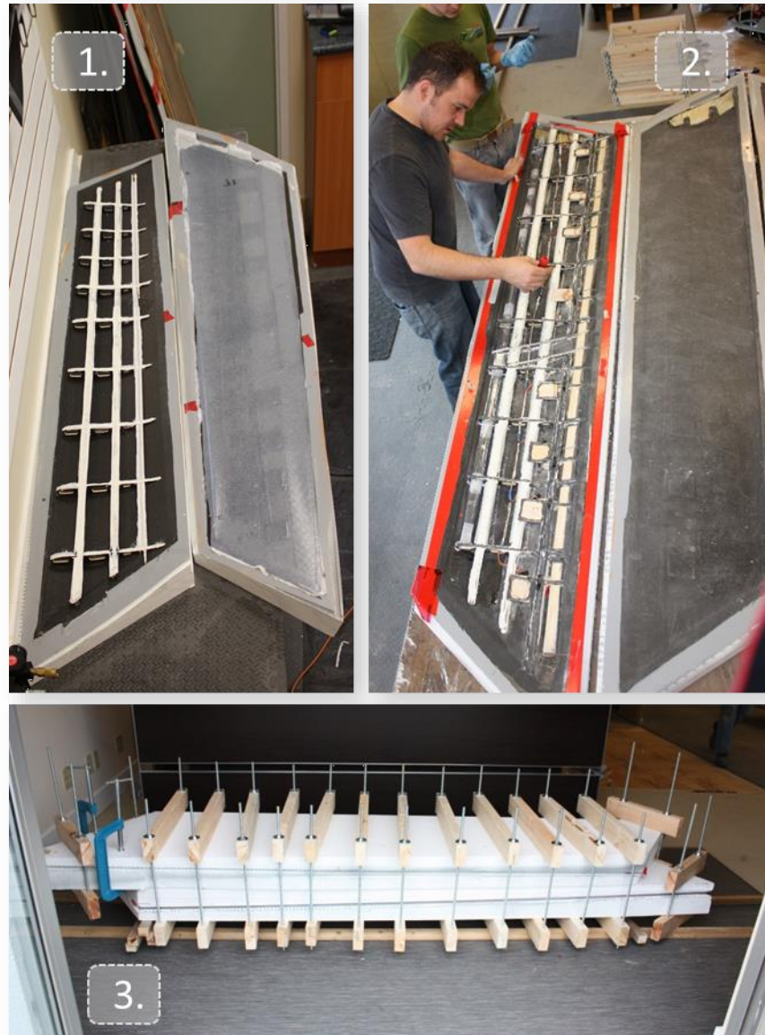
FIGURE 69 - ASSEMBLY OF WING STRUCTURE
