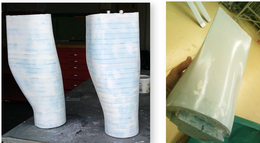
FIGURE 65 - MALE PLUGS USED FOR PRODUCING AIR INTAKE SKINS (LEFT) AND OUTLET SKINS (RIGHT)
