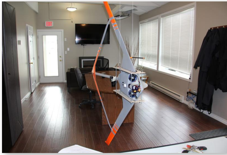
FIGURE 151 - BIFILAR PENDULUM TEST IN PITCH AXIS
