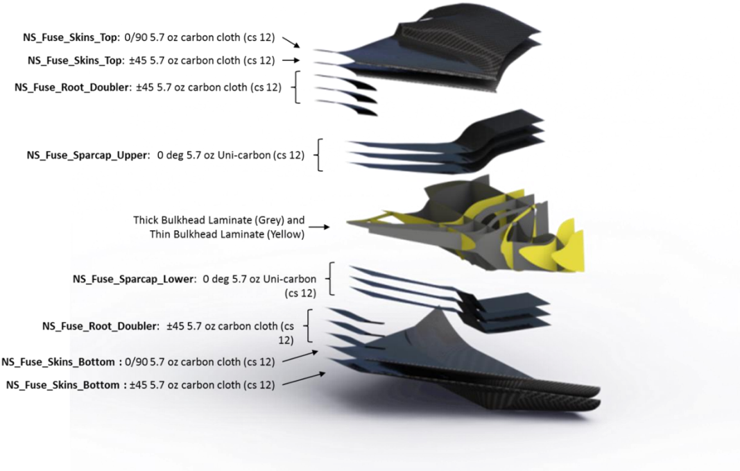
FIGURE 41 - FUSELAGE LAYUP
