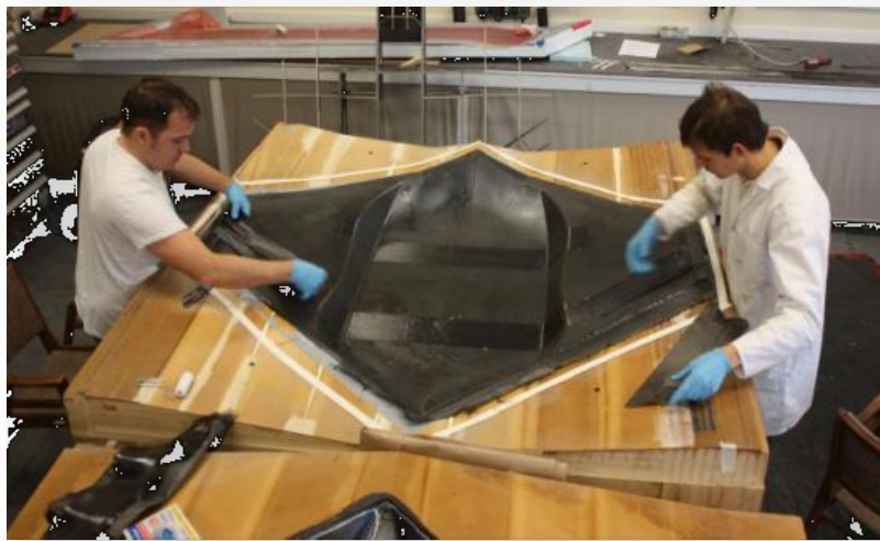
FIGURE 66 - LAYING UP BOTTOM FUSELAGE SKIN
