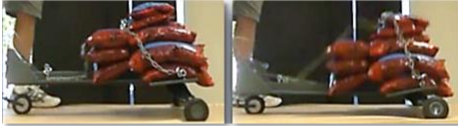
FIGURE 77 - LANDING GEAR AT IMPACT (LEFT); LANDING GEAR AFTER TEST (RIGHT)
