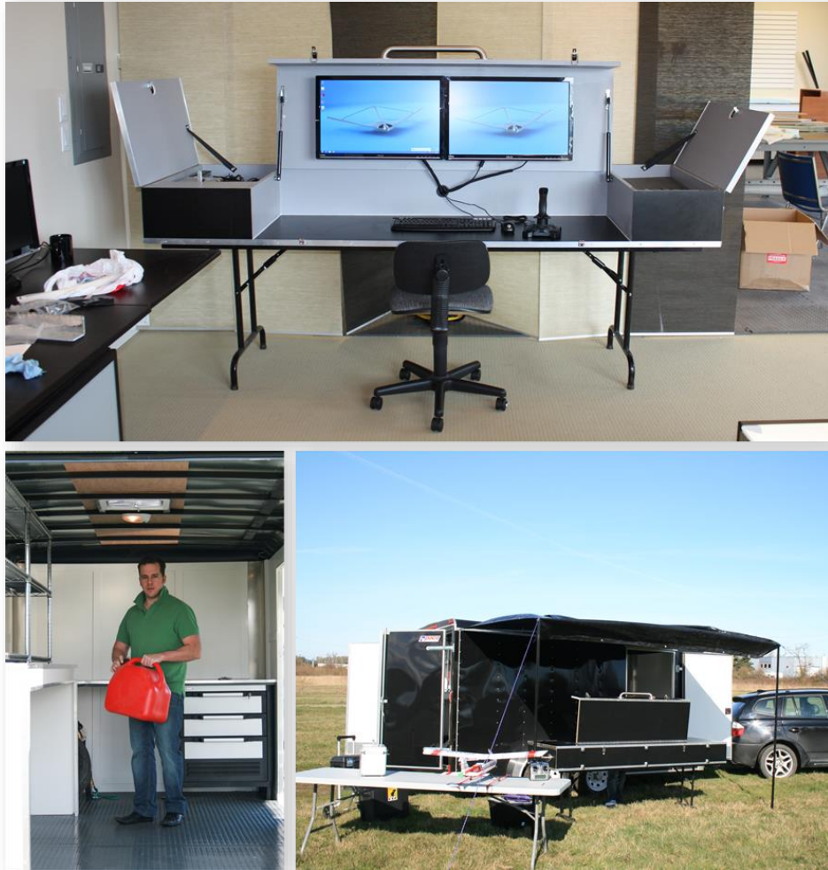
FIGURE 56 - INITIAL MOBILE COMMAND CENTER: COMPUTER STATION (TOP AND LOWER RIGHT), INTERIOR OF CUSTOM TRAILER (LOWER LEFT) AND DEPLOYED SETUP (LOWER RIGHT)
