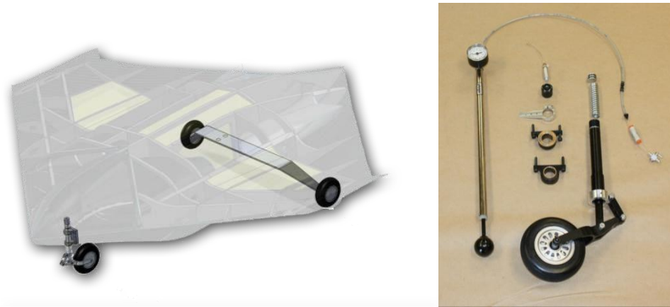
FIGURE 48 - TRICYCLE LANDING GEAR LAYOUT AND CUSTOM OLEO STRUT
