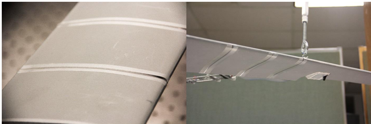
FIGURE 117 - GAP SEALING TECHNIQUES (LEFT SHOWS FLEXIBLE TAPE AND RIGHT SHOWING LAP JOINT USING HINGE TAPE)
