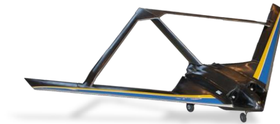
FIGURE 50 - MINI SENSORCRAFT USED TO EVALUATE PROPOSED LANDING GEAR GEOMETRY
