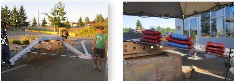
FIGURE 75 - STATIC LOADING OF AIRCRAFT
