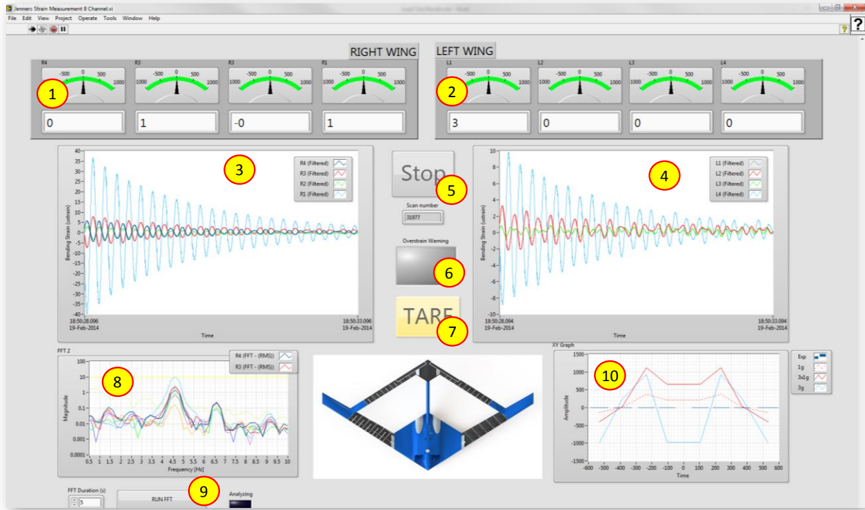
FIGURE 133 - CUSTOM INTERFACE FOR CALCULATING, FILTERING AND DISPLAYING MEASURED STRAIN
