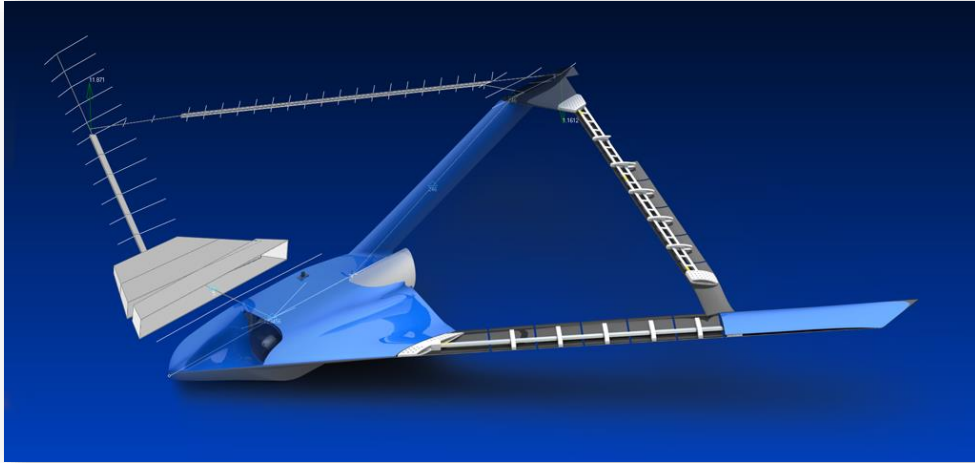
FIGURE 141 – FE MODEL OF SENSORCRAFT CONFIGURATION SHOWING UPDATED TAPED BEAM INBOARD WING SECTIONS
