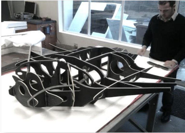
FIGURE 63 - INTERNAL STRUCTURE OF RIGID RPV FUSELAGE
