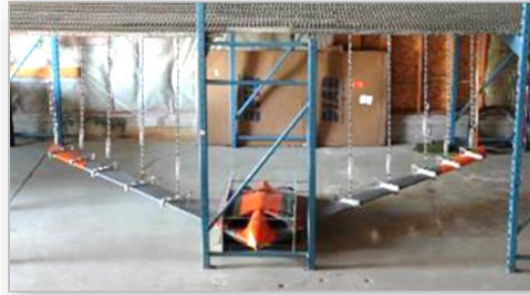
FIGURE 76 - IMPROVED STATIC LOADING RIG SHOWING LOADING OF FRONT WINGS
