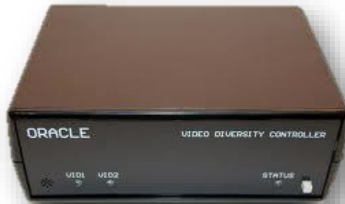
FIGURE 55 - VIDEO DIVERSITY SWITCH USED AT GROUND STATION
