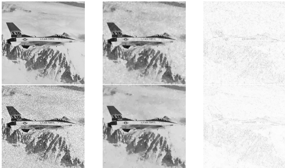
Figure 5.6: Denoising jet (up to bottom, left to right) (a) original image (b) noisy image (c) denoised image by the TV-l_1 (d) denoised image by the IRTV (e) difference image between the TV-l_1 denoised image and original image (f) difference image between the IRTV denoised image and original image
