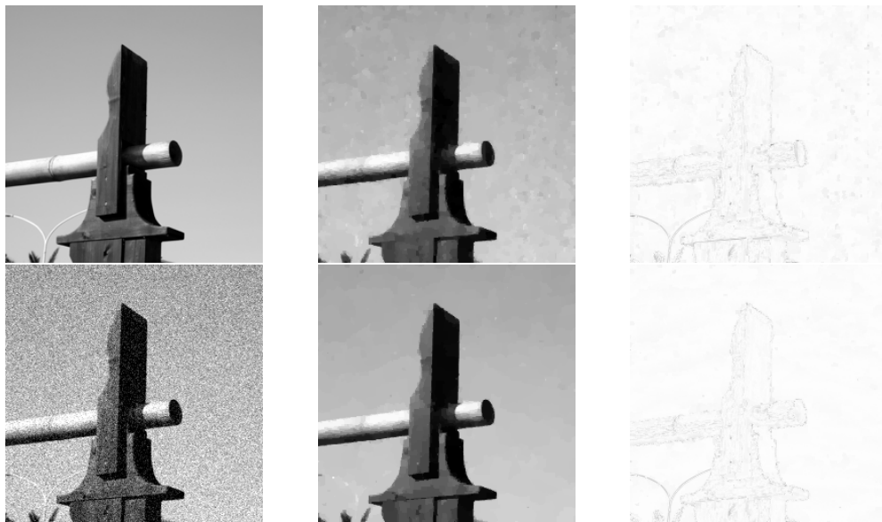
Figure 5.4: Denoising axe (up to bottom, left to right) (a) original image (b) noisy image (c) denoised image by the TV-\ell_1 (d) denoised image by the IRTV (e) difference image between the TV-\ell_1 denoised image and original image (f) difference image between the IRTV denoised image and original image
