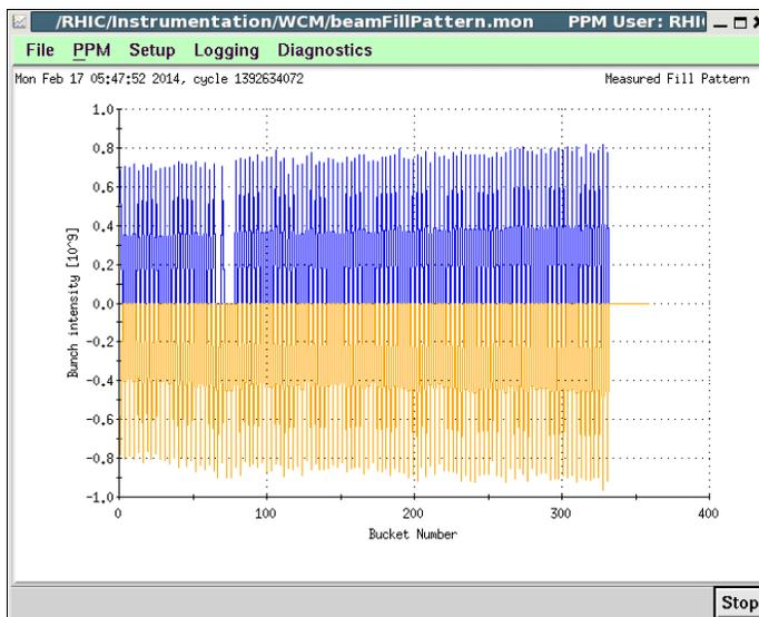
**Figure 3.8:** Bunch fill pattern in all RF buckets measured by the WCMs.
