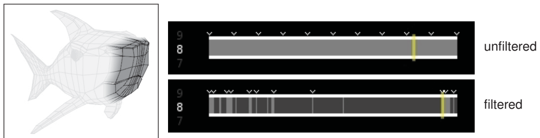
Figure 2.3: User interface. A large view shows the mesh of the current cluster. Across the bottom is the timeline with indicators of the current cluster and any filtered clusters. The thumbnails show changes at different places along the timeline.
