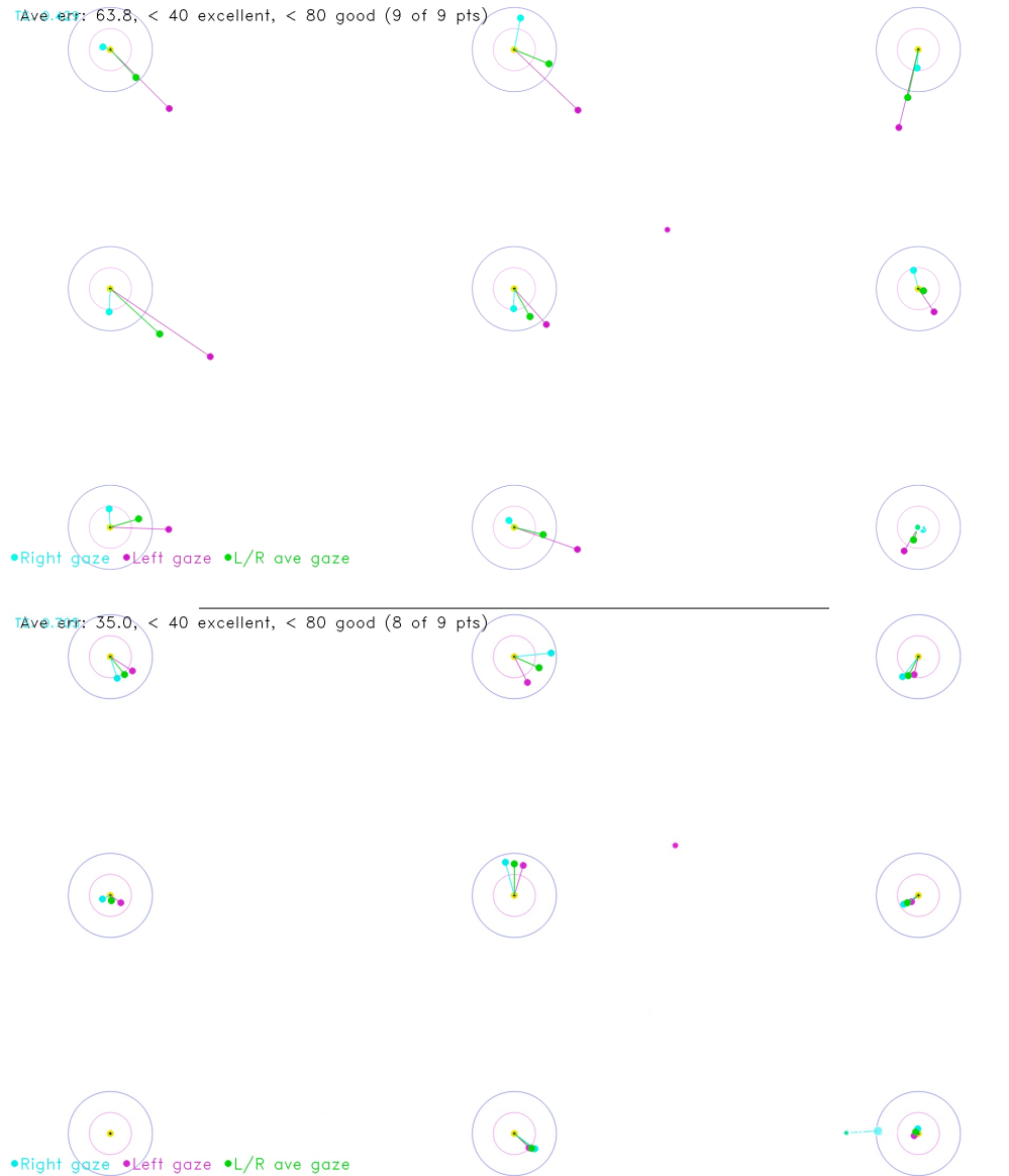
Figure 2.2: Eye-tracking calibration results for (a) a user with poor accuracy near the corners of the screen and (b) a user with poor accuracy near the centre of the screen
