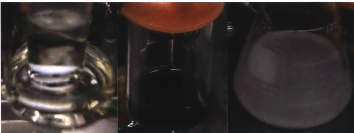
Figure A.16. Vial of 6 and \text{Fe}(\text{BIPhMe})\text{Cl}_2 (left). After addition of (\text{PPN})(\text{SSNO}) to the solution of 6 , \text{NO}(\text{g}) is released and converts \text{Fe}(\text{BIPhMe})\text{Cl}_2 to [\text{Fe}(\text{BIPhMe})_2(\text{NO})\text{Cl}][\text{Fe}(\text{NO})\text{Cl}_3] (middle) and \text{Zn}\{\text{S}\} (right).
