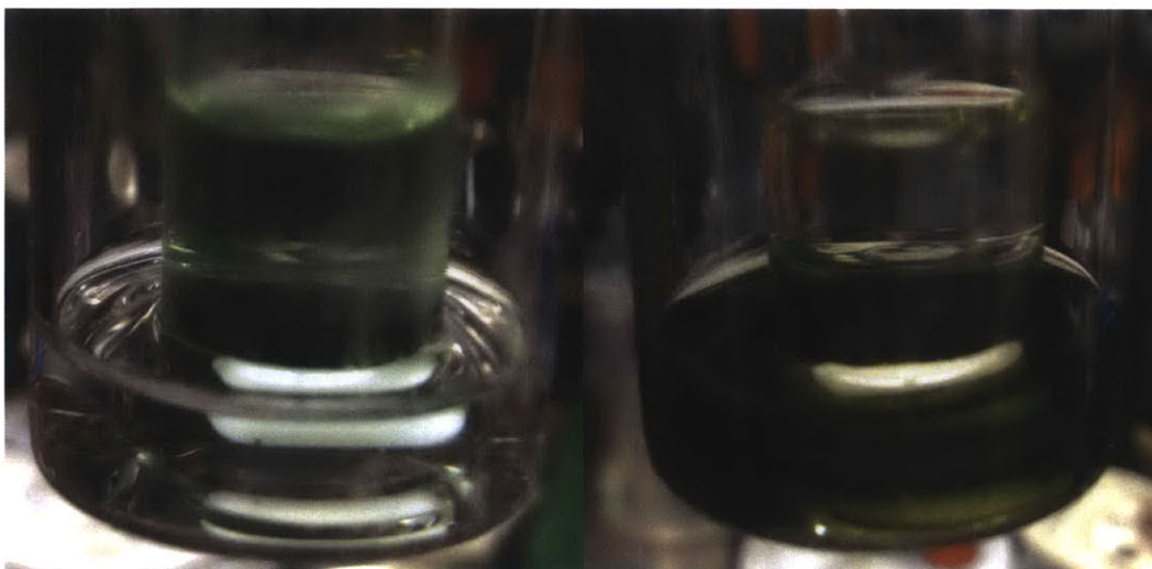
Figure 3.8. Left: A 20 mL vial containing a colorless solution of 8 in acetonitrile and a 5 mL vial containing a green solution of 2 in acetonitrile. Right: Addition of 3 to the solution of 2 results in color loss by decomposition of \text{SNO}^- to form \text{NO}(\text{g}) . The released \text{NO}(\text{g}) reacted with the solution of 8 to turn it green.
