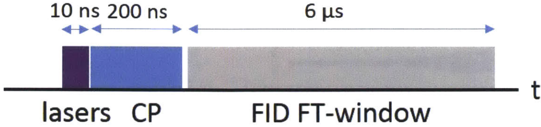
Figure 3-9: Schematic diagram of time-sequence in CPmmW-FID experiment. The timing values in this figure are for typical experiments. The gap of lasers and chirped pulse is \sim 10 ns, and the gap of the chirped pulse and FID FFT window is \sim 30 ns.
