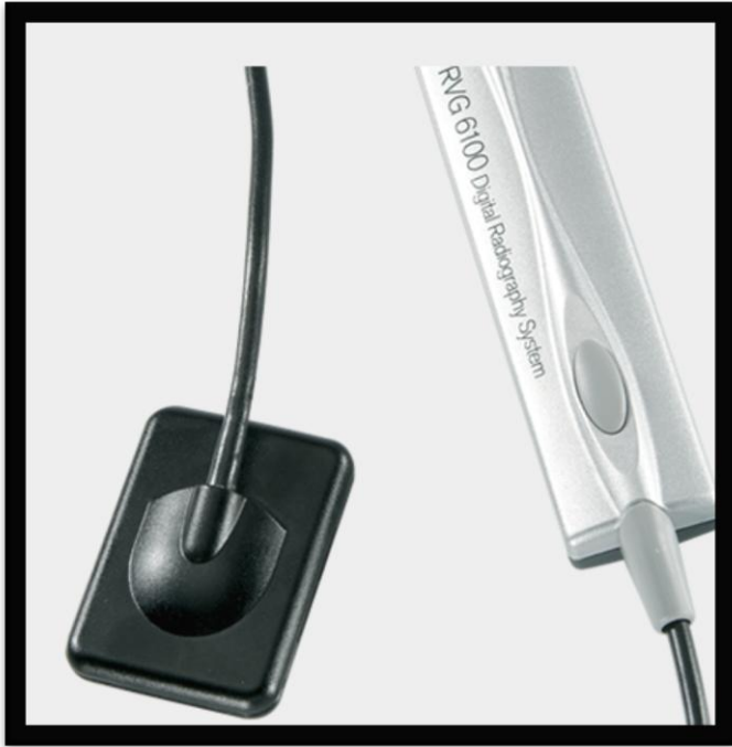
Figure 2-1. Carestream Dental Systems RVG 6100 Direct Capture Sensor (Figure Source: http://mediaroom.carestreamdental.com/press-materials/image-galleries/digital-intraoral-sensors/rvg-6100 )
