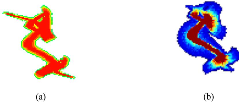
Figure 4.4. (a) Simulation result on model from Figure 4.3, showing the saturation of CO<sub>2</sub> after 3 years of injection. (b) Result of proxy run for the same model.
