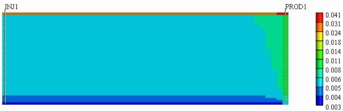
Figure 4-23: Gas saturation after 70 years for k_v/k_h = 1.0 .
