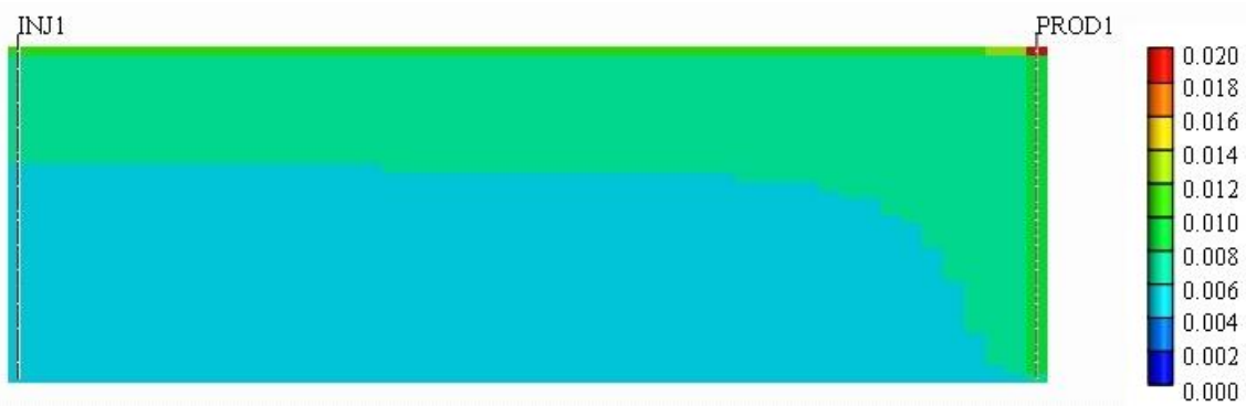
Figure 4-22: Gas saturation after 70 years for k_v/k_h = 0.1 .
