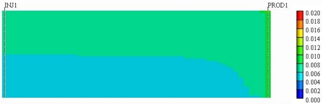
Figure 4-21: Gas saturation after 70 years for k_v/k_h = 0.01 .
