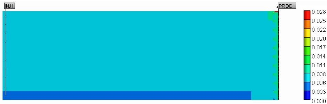
Figure 4-20: Gas saturation profile on a vertical cut between injector and producer at 20 years. Injector is shut in.
