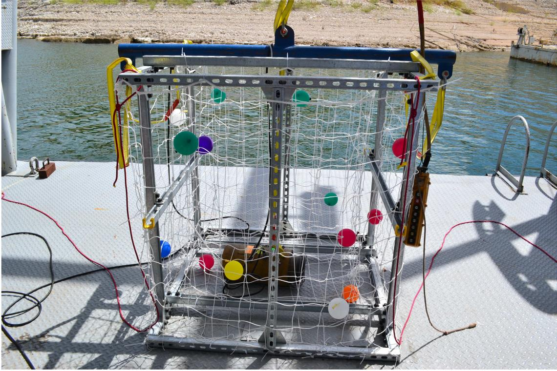
Figure 4.5: Photo of unistrut cage and nylon netting used to attach balloons.
