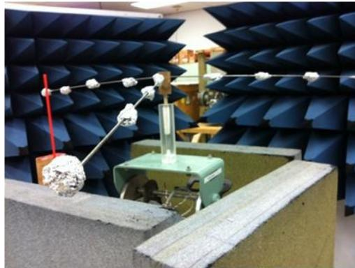
Figure 4.7: Measurement set-up to cause physical in-plane vibrations.
