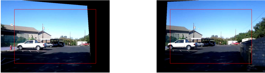
Figure 1.5: Illustration of the black border problem. Black border intrudes into the cropping window in the left image, but not in the right image.
