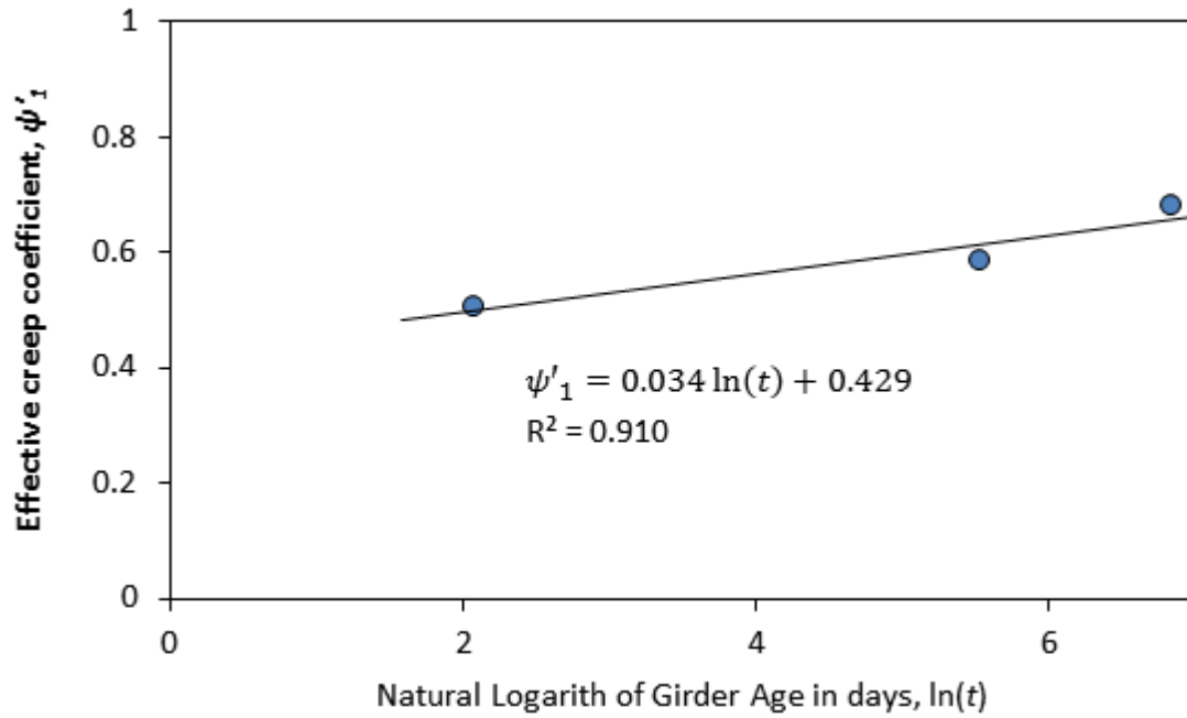
Figure B-10 Effective creep coefficient in terms of time for Girder UTPS#232 (II-3)
