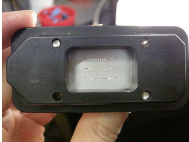
Figure 2.30: CXRS 90 \mu\text{m} slits and dissector. The fibers have been backlit from the breakout box.
