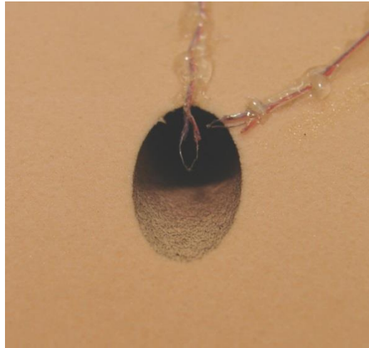
Figure 0-7 Photograph of a thermocouple installed at the coolant hole entrance.
