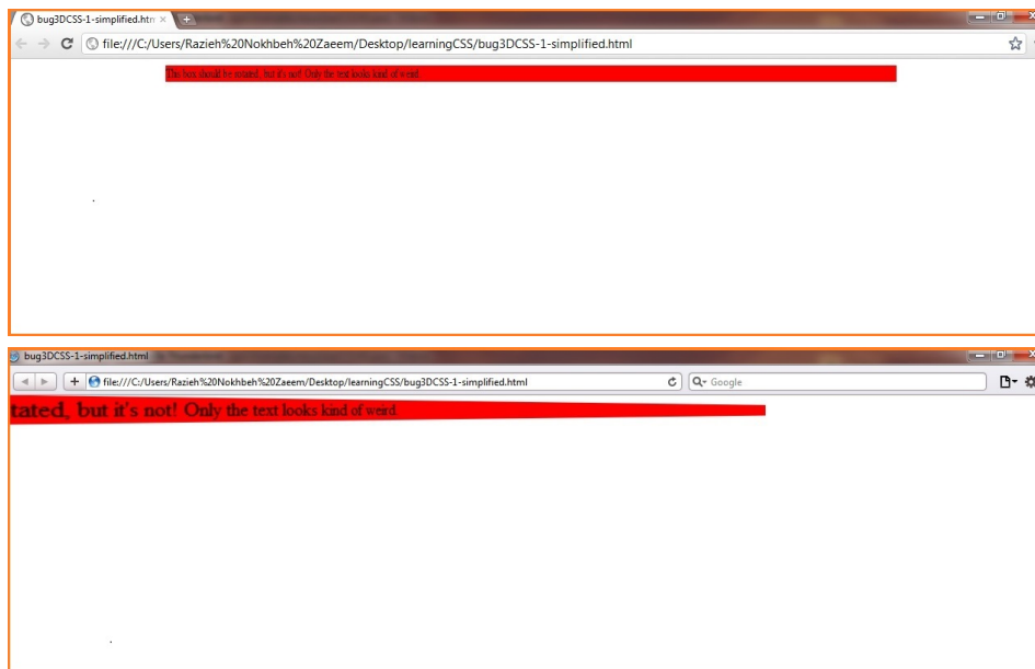
Figure 6.14: A webkit-perspective bug found in Chrome (up). Safari (down) shows the expected output.
