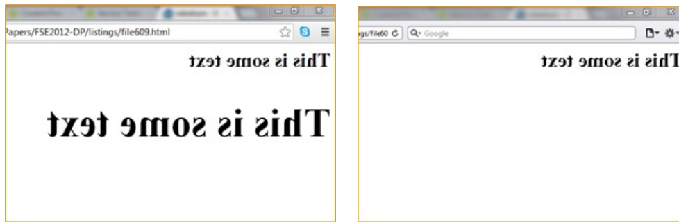
Figure 6.13: A back-face visibility bug found in Chrome (left). Safari (right) shows the expected output.
