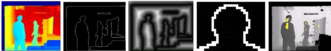
Figure 3.2: Intermediate results of 2D Chamfer distance matching. (a) Preprocessed depth image. (b) Binary edge image calculated by Canny edge detector. (c) Distance map generated from binary edge image (d). The binary head template (e). 2D template matching result (yellow dots indicate the detected locations).
