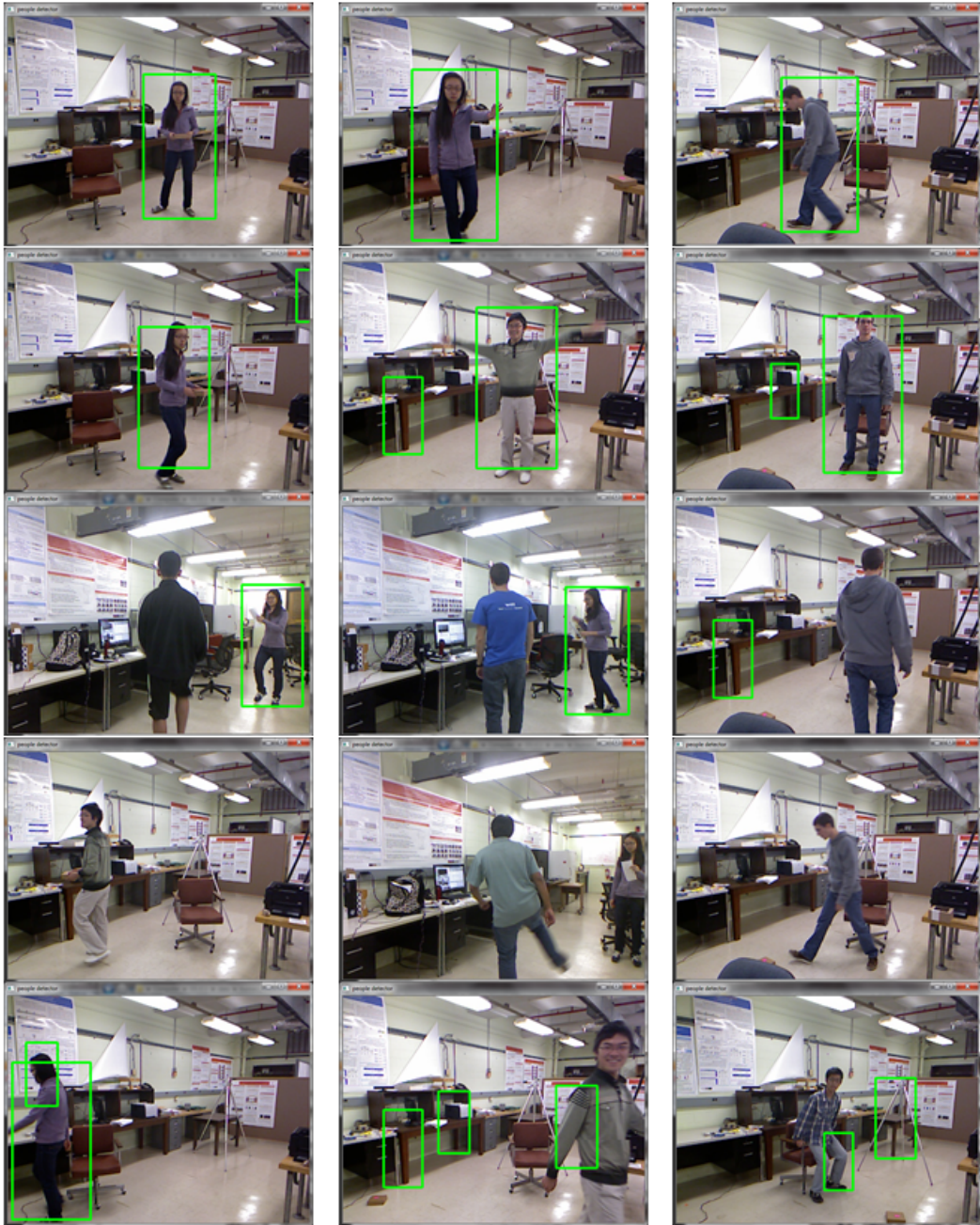
Figure 3.9: Detection Results using HOG pedestrian detection algorithm.
