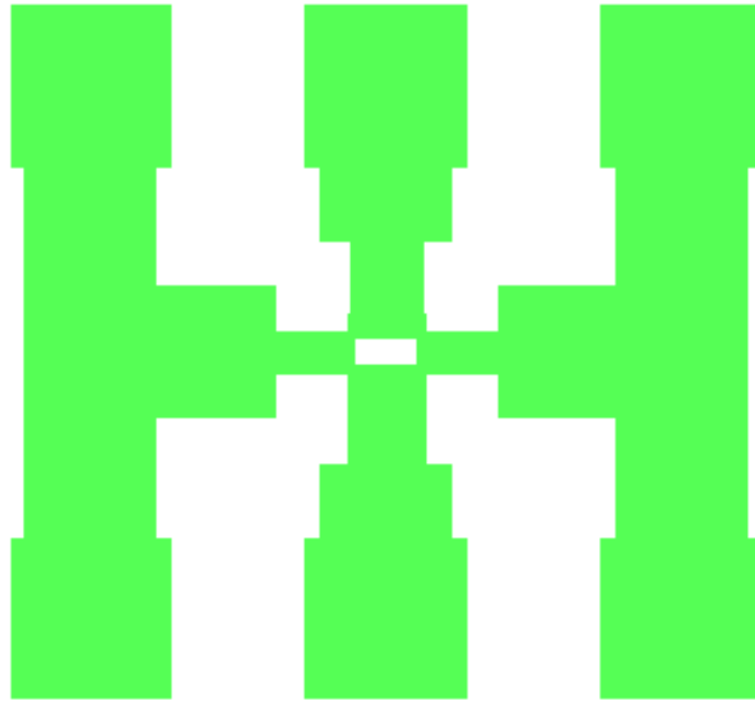
Figure A.9. Mask3 for Multi-finger Embedded-gate Graphene Field-Effect Transistors to define graphene active areas.
