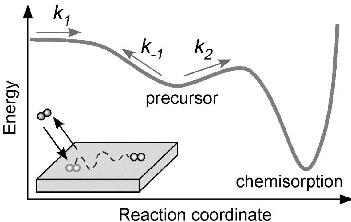
**Figure 1.1.** Schematic potential energy surface for the chemisorption of small molecule on a solid surface.
