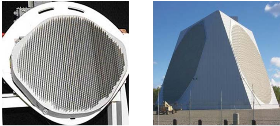
Figure 4-1: Example of phased array antennas. AN/APG-77 F-22 Radar [64] (left) and PAVE PAWS Radar at Clear AFS, Alaska [63] (right).
