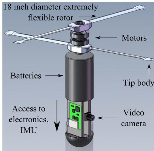
Figure 1.2: Micro-helicopter with 18 inch diameter flexible rotors
