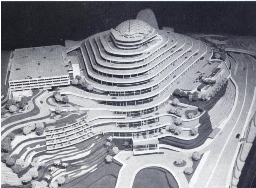
FIGURE 11.13 J. Romero Gutiérrez, P. Neuberger, and D. Bornhorst, the Helicoid, Caracas, 1955-1959. Two different stages of the project. The first one (1955) showed a sort of “Nervi” structure at the top, with a “mini-helicoid” for pedestrians. The second version (ca. 1959) exhibited the Fuller’s dome atop the building, an enlarged parking area (Parking Building, on the left), and a landscape treatment in front of it. Source: Werner G. Krug, Orion 5, 1959, 385.
