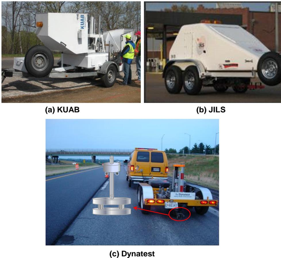
**Figure 6. Examples of FWDs from KUAB, JILS, and Dynatest.**
