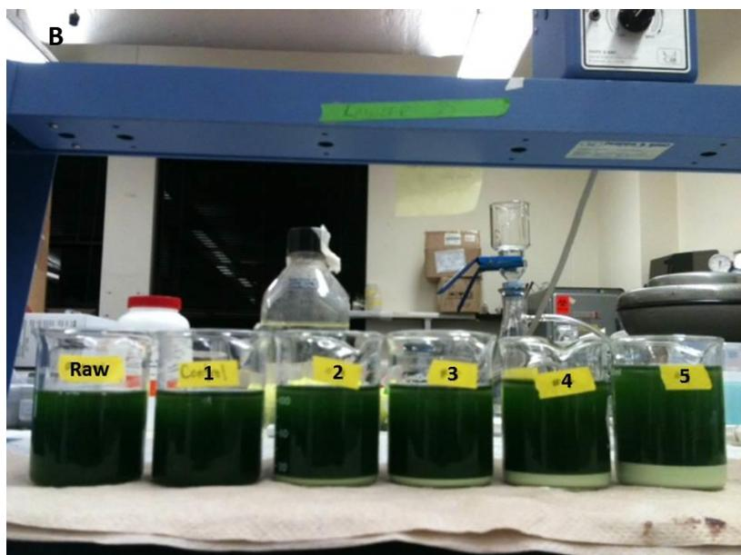
Figure 5-4 Effect of calcium carbonate dose (pre-precipitated  $\text{CaCO}_{3(s)}$ ) addition on algae removal efficiency for a range of algae cell densities (panel A). The pH of the solutions was maintained at 10.6. The image (panel B) represents the test results after sedimentation for an algae cell density of 2.0 g/L. “Raw” represents the untreated original solution and the numbers represent doses of 0, 7000, 14000, 28000, and 57000 mg  $\text{Ca}^{2+}$ /L, respectively from 1 to 5.
