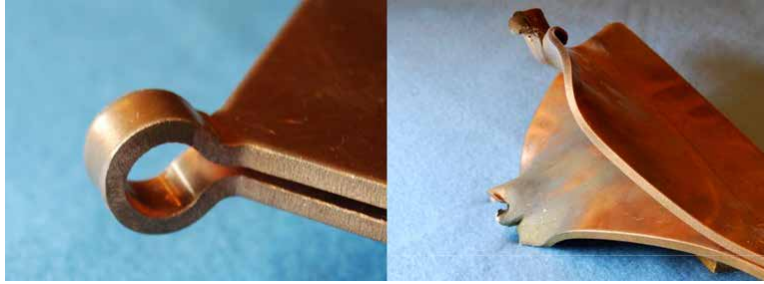
Figure 2.1: Left to right, a high-field ( \sim 200 T) coil before and after a shot. Magnetic pressure within the copper loop explodes the coil. Images courtesy of C. Mielke, LANL [57].
