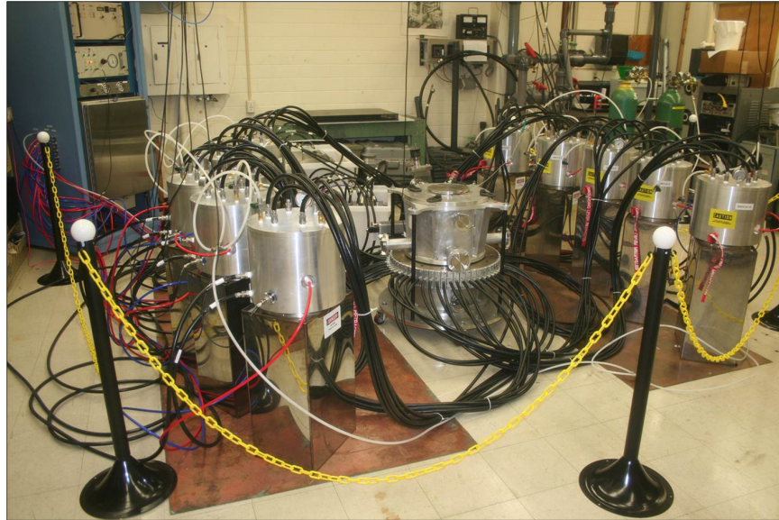
Figure 3.3: The entire MegaGauss 2 system at The University of Texas at Austin. All ten capacitors are connected to the central vacuum chamber. The control electronics rack and charge and trigger distribution tanks are visible in the background.
