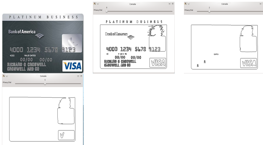
Figure 5.3: Output of the sketching transform on a credit card image at different privacy levels.
