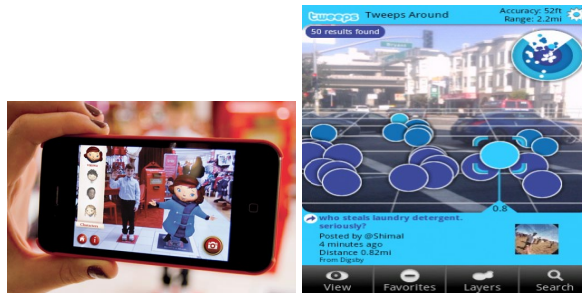
Figure 4.2: Two examples of mobile perceptual applications that only need specific objects in a sensor stream. On the left, Macy’s Believe-O-Magic only needs the location in the frame of a special marker, on top of which it renders a cartoon character. On the right, Layar only needs to know the GPS location and compass position to show geo-tagged tweets.
