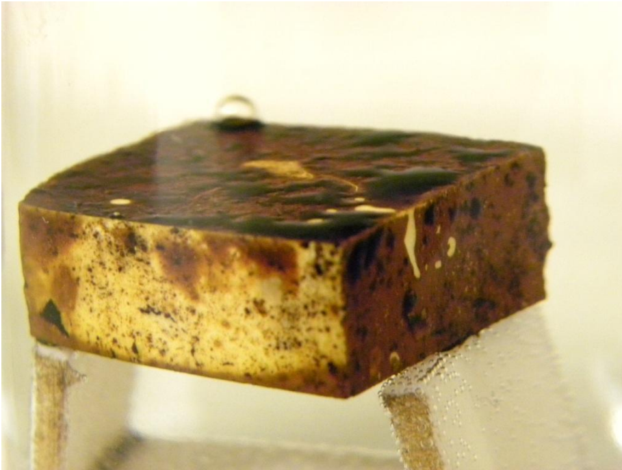
Figure 5-10: Photograph of cristobalite plate in formation brine after aging.
