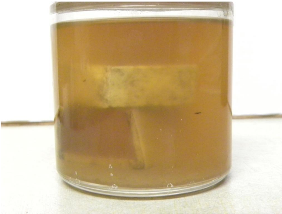
Figure 5-11: Photograph of cristobalite plate in surfactant solution at optimum salinity.
