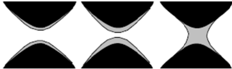
Figure A3: Scheme of liquid accumulating in a pore throat
