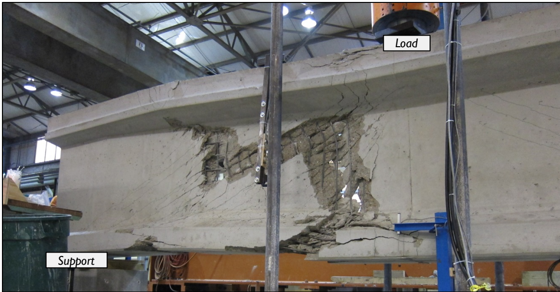
Figure 4-17: Failure of Control Specimen, Tx62-3(S)
