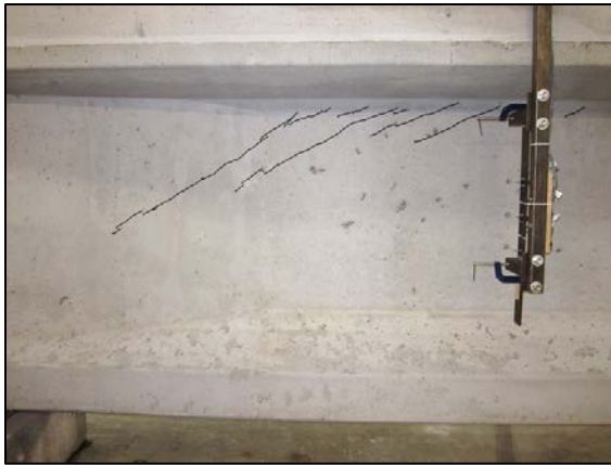
(A) Tx62-3(S): Control Girder First Cracking at V_{FD} = 0.41V_{test}
