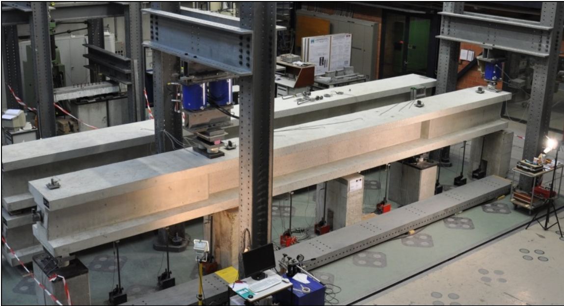
Figure 2-20: Test Setup of Rupf, Ruiz, & Muttoni (2013) (Muttoni, 2014)
