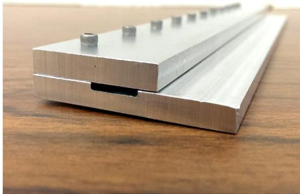
Fig. 5.6 The prototype of the proposed two-section microstrip LWA consists of two aluminum blocks. The air-filled region is removed from the bottom ground plane using a milling machine and the top aluminum block works as the top microstrip.
