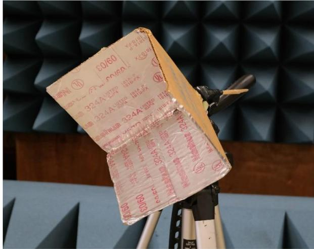
Fig. 3.9 The trihedral target, which is 16cm per side.
