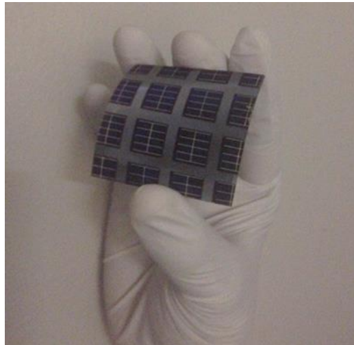
Figure 3.7: A completed single heterojunction (SHJ) solar cell on 2 inch square substrate. The individual blue squares are isolated devices.
