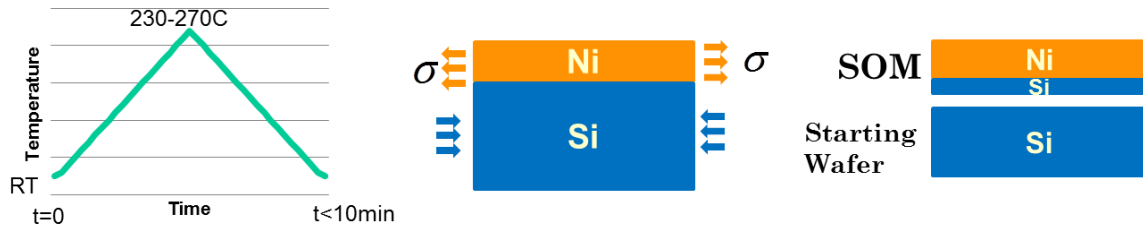
Figure 2.2: Schematic of the exfoliation process flow.
