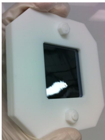
Figure 3.5: Custom made exfoliated substrate holder used for uniform KOH texturing.
