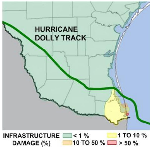
Fig. 2.8. Power infrastructure damage intensity caused by Hurricane Dolly.
