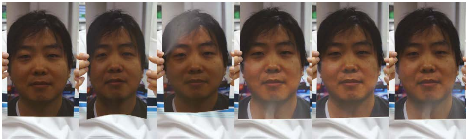
Fig 13. Example sequence of a warped photo attack from the CASIA FASD (Zhang et al. 2012). This describes the characteristic reflections (flickering) of a planar spoofing medium and the distorted motion patterns. Paper V © Springer.
