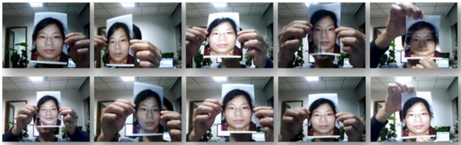
Fig 3. Attack samples from the NUA Photo Imposter Database by Tan et al. (2010). Vivid photo attacks are simulated by translating, rotating and bending (warping) a photograph.
