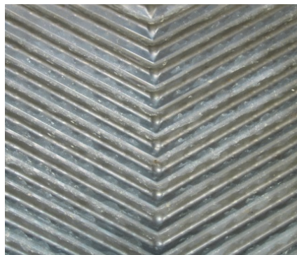
Fig. 3. Corrugated heat transfer surface of a plate heat exchanger.
