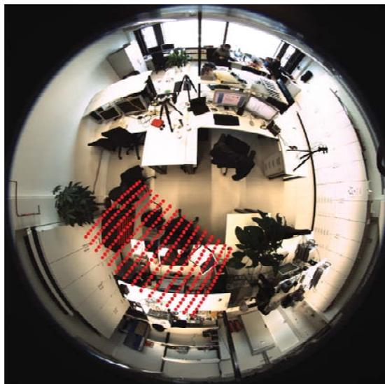
**Figure 4.11:** Projection of sub-sampled 3D camera coordinates to 2D source image coordinates
