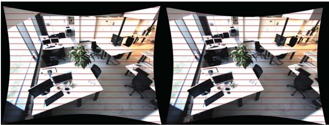
Figure 3.4: Rectified images with exemplary epipolar lines
