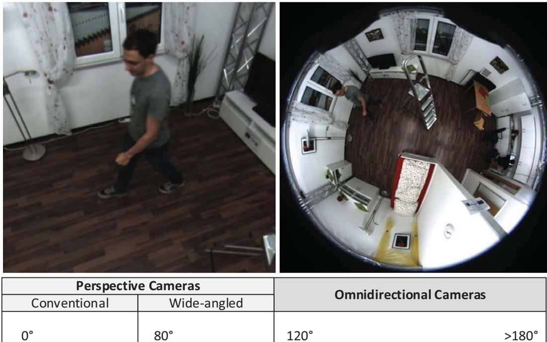
**Figure 1.5:** Standard perspective camera versus omnidirectional camera in a home environment
