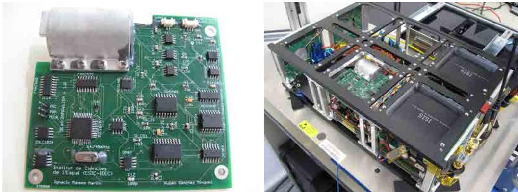
Figure E.4: Flight model of the eLISA-AMR payload for the <sup>3</sup>Cat-2 mission. Right: payload integration of the flight model in the CubeSat.
