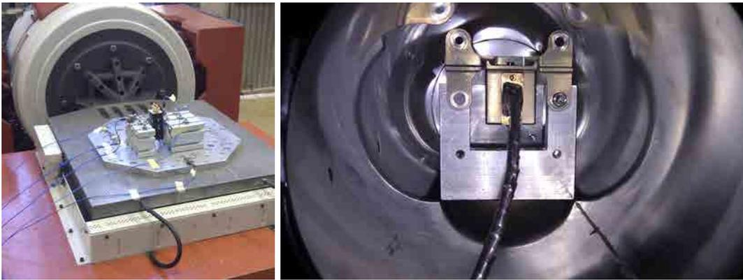
Figure 2.11: Vibration test facility and degaussing process. Left: the flight model fluxgate magnetometer under test is placed on the table structure in front of the shaker system. Right: the magnetometer is fixed onto an aluminum support and placed inside a magnetic shielding for degaussing purpose after the vibration test.
