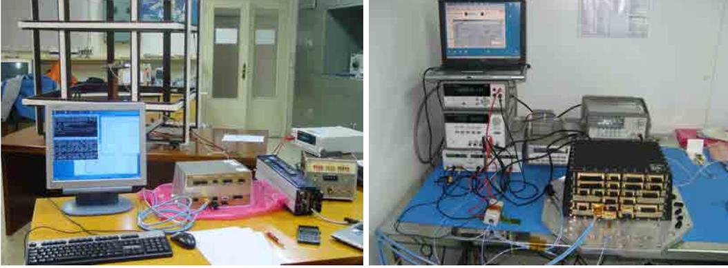
Figure 2.7: Test facility for measuring the range and uncertainty of the magnetic measurement subsystem. Left: engineering model test including the DMU and the magnetometer (in the center of the three-axis coil system). Right: test of the flight model DMU using simulated magnetometer readings.
