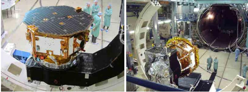
Figure 2.9: On-station thermal test campaign. Left: LISA Pathfinder at the IABG mbH facilities during the OSTT test. Right: The spacecraft in front of the space vacuum chamber. Credits: Airbus DS.
