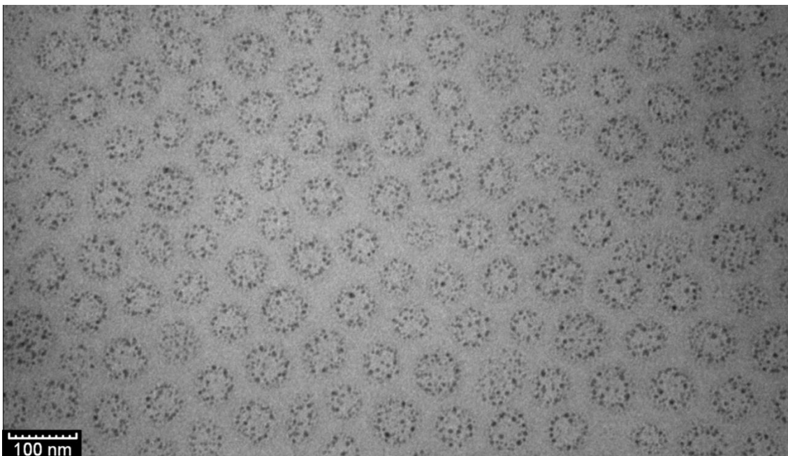
Figure 3.10. TEM image of PS- b -P4VP micelles with the incorporation of Au 3+ at Au 3+ /P4VP ratio of 10:1. The sample was prepared by spin-coating PS- b -P4VP/HAuCl 4 micelles at 3000 rpm/min.
