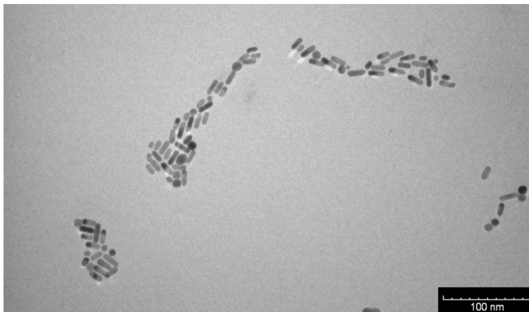
Figure 7.13. TEM image of short Au nanorods formed at the low \text{Ag}^+ concentration (i.e., 0.04 mM) without the addition of toluene.
