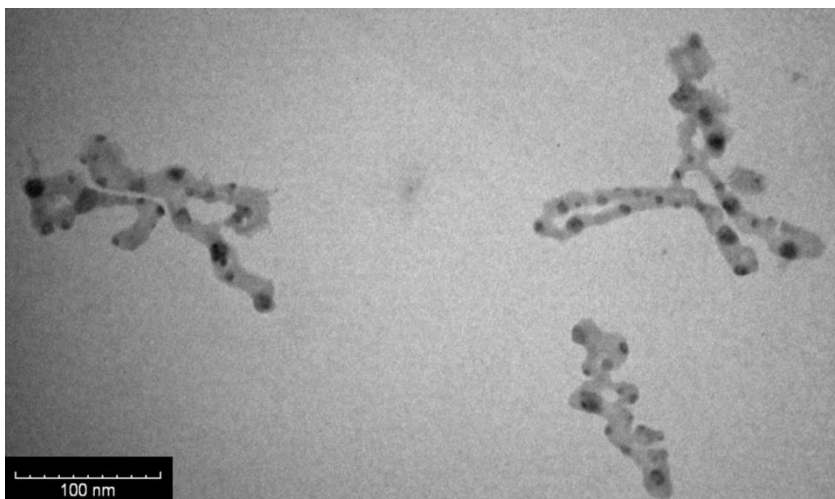
Figure 7.11. TEM image of Au nanostructures with irregular shapes formed at low \text{Ag}^+ ion concentration (i.e., 0.04 mM by adding 40- \mu\text{l} 0.01M \text{Ag}^+ solution to a 10-ml Au growth solution) with the addition of 100- \mu\text{l} toluene. The concentration of CTAB was 0.1M.
