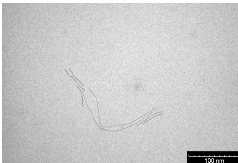
Figure 7.17. TEM image of ultrathin Au nanowires formed by adding a 80\text{-}\mu\text{l} chloroform to the Au growth solution after adding the Au seed solution. The growth solution was prepared by mixing 10 \text{ ml} 0.1 \text{ M} CTAB aqueous solution with 0.5 \text{ ml} 10 \text{ mM} \text{HAuCl}_4 , 40 \mu\text{l} 0.1 \text{ M} \text{AgNO}_3 and 0.5 \text{ ml} 0.1 \text{ M} hydroquinone aqueous solution.
