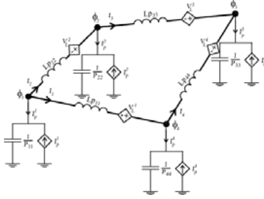
Figure 9: (L_p, P, \tau) PEEC model for metal patch in Fig. 8 discretized with four edge nodes. Controlled current sources, I_p^n , account for the electric field coupling and controlled voltage sources, V_L^n , account for the magnetic field coupling.
