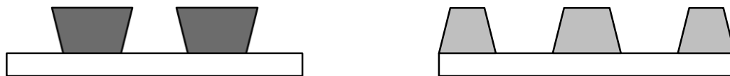
Figure 1.8: Illustration of sidewall profiles of negative tone (left) and positive tone (right) materials
