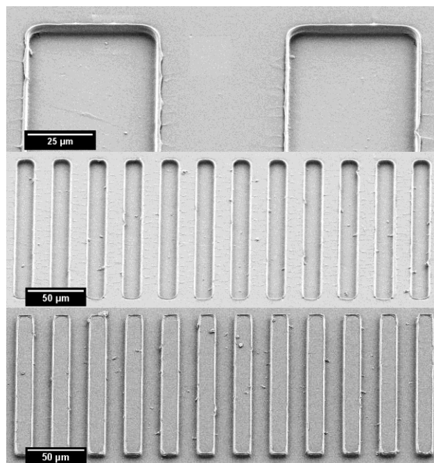
Figure 8.13: SEMs of 50 \mu\text{m} trenches (top), 16 \mu\text{m} trenches (middle), and 16 \mu\text{m} hills (bottom)
