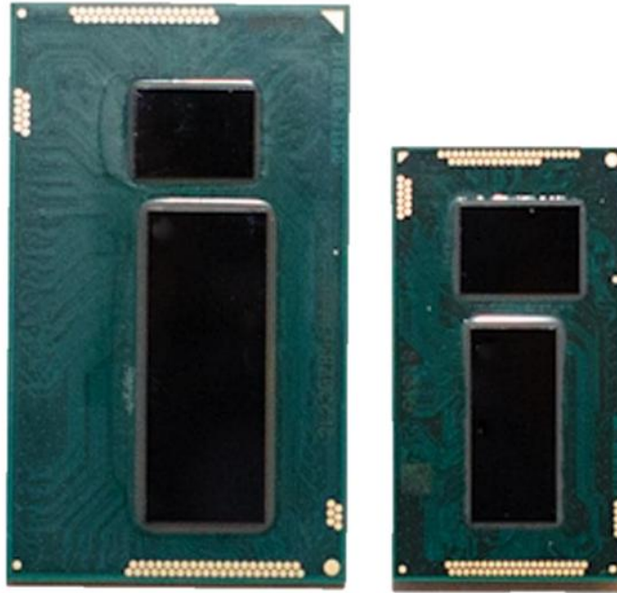
Figure 1.1: Evolution of Intel chip package from 4 th (left) to 5 th generation (right) © 2014 Intel Corporation. Used with permission [1]
