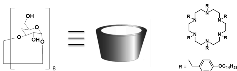
Figure 1.4 First reported fullerene receptors: \gamma -cyclodextrin and azacrown-based receptor. 26, 27
