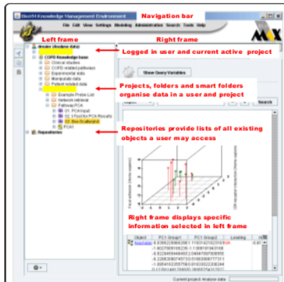
Figure 6 BioXM graphical user interface overview. The BioXM graphical user interface (GUI) consists of three frames. A Navigation bar provides the functions for importing, managing, reporting and searching data. A project and repositories frame to the left, allows all data available to a user to be accessed in the repositories section and the data to be organised in a user and project specific way in the projects section. A right frame, is used to display detailed information about any object selected in the left frame.
